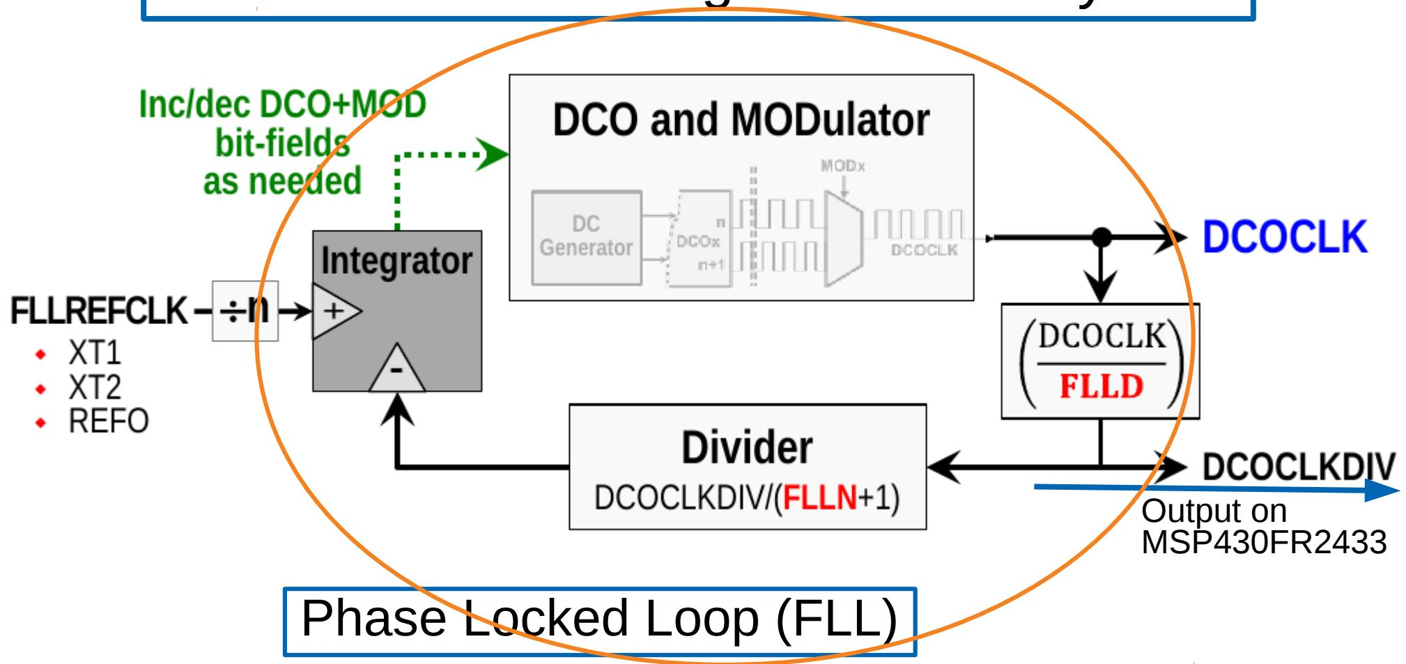
Figure 3-1. Clock System (CS)
