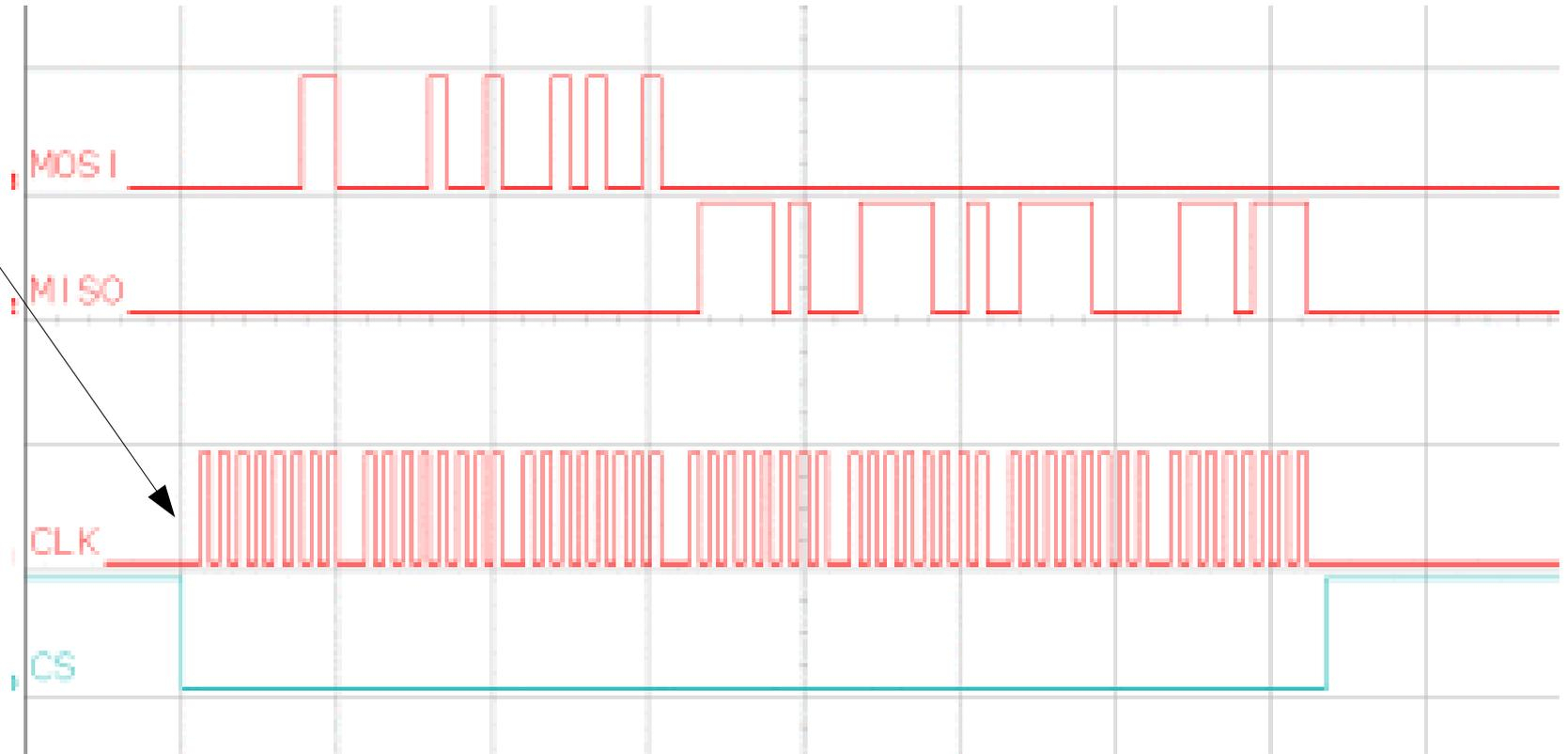
3. The master keeps cycling the clock, bits are traded, and after eight bits, both sides read in the received data and queue up the next byte for transmission.
