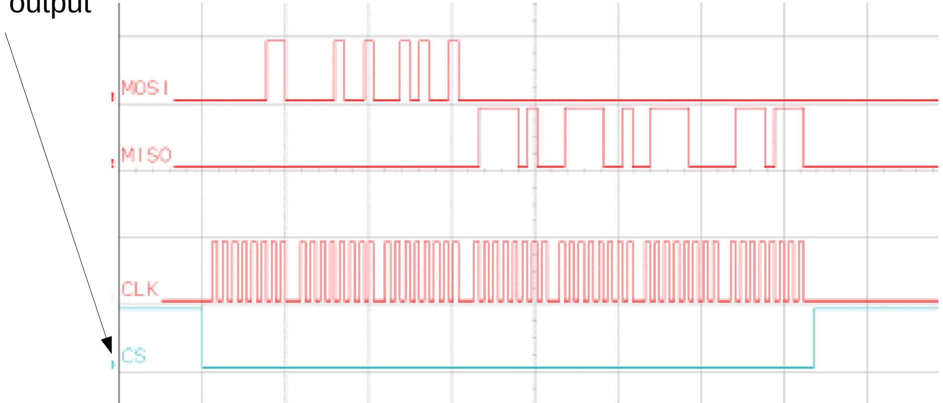
2. The master sends the first clock pulse and the first bit of data moves from master to slave (along MOSI) and from slave to master (along MISO).
