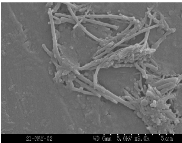
Figure 24. MWNT lengths after mechanical grinding with mortar and pestle.
