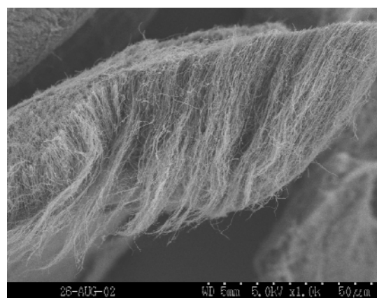
Figure 4. MWNTs from CVD synthesis based on ferrocene and xylene at 1023 K.
