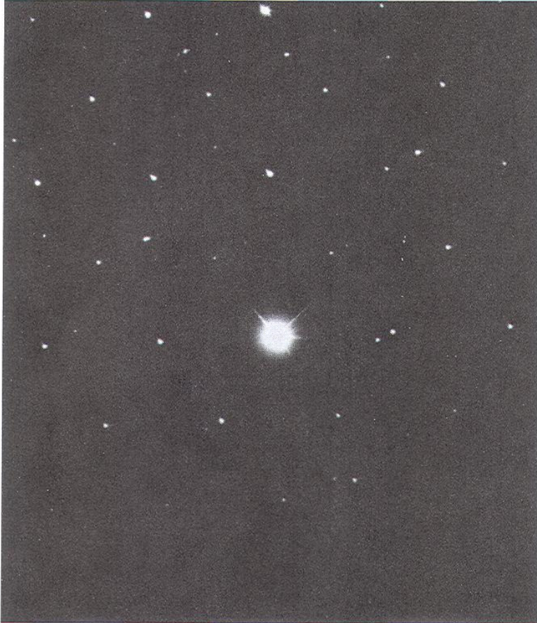
Figure 11.1. An experimentally observed diffraction pattern showing the central, intense, direct beam and an array of diffraction spots from different atomic planes. Such a pattern, with sharply focused spots, is best obtained by underfocusing the beam.
