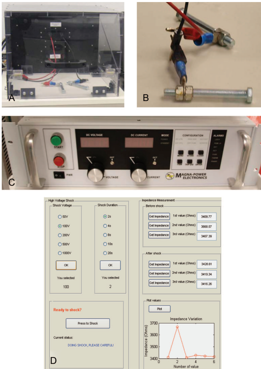
Figure 1. Electrical burn delivery system. Plexiglass exposure chamber that is totally enclosed with ventilation fan and safety alarm that sounds upon opening (A); contact electrodes (B); power supply (C); screenshot of the control application illustrating the user interface (D).
