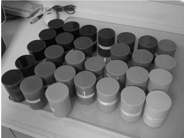
Fig. 8. Picture of the phantom grid. Absorption coefficient \mu_a increases from bottom row to top row whereas reduced scattering coefficient \mu'_s increases from left column to right column.
