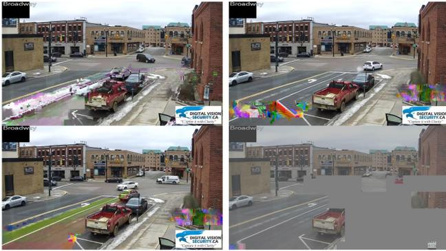
Fig. 15. Exemplary artifacts occurring when transmitting H.265 encoded streams (DVS dataset [31]) via a wireless connection at a packet loss rate of 0.1% after MAC layer BEC.
