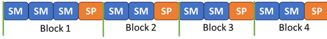
Fig. 7. CenterPoint's 3-D backbone broken into blocks. SM: submanifold sparse convolution. SP: sparse convolution.
