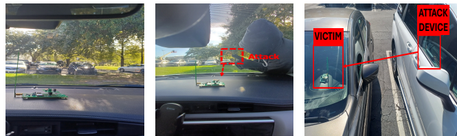
(a) User Case: An energy harvesting device is placed underneath a vehicle’s windshield (b) Attack Case 1: Adversaries degrade a victim capacitor remotely outside of the vehicle. (c) Attack Case 2: Adversaries degrade a victim capacitor remotely from another vehicle.
