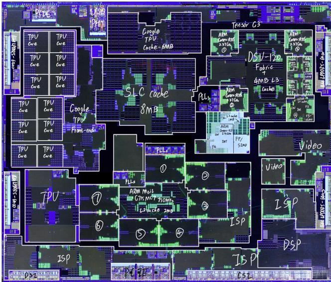
Fig. 1: Chip Layout for Google Tensor G3 [14].
