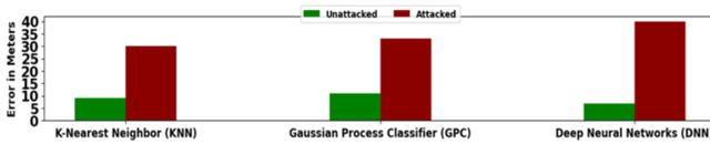
Fig. 1. Impact of rogue APs on three popular ML-based indoor localization solutions [15], [16], [17] from prior work.
