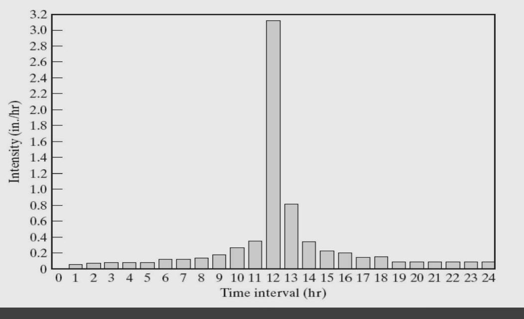
Figure : SCS type II , 5-yr 24-hr design storm
