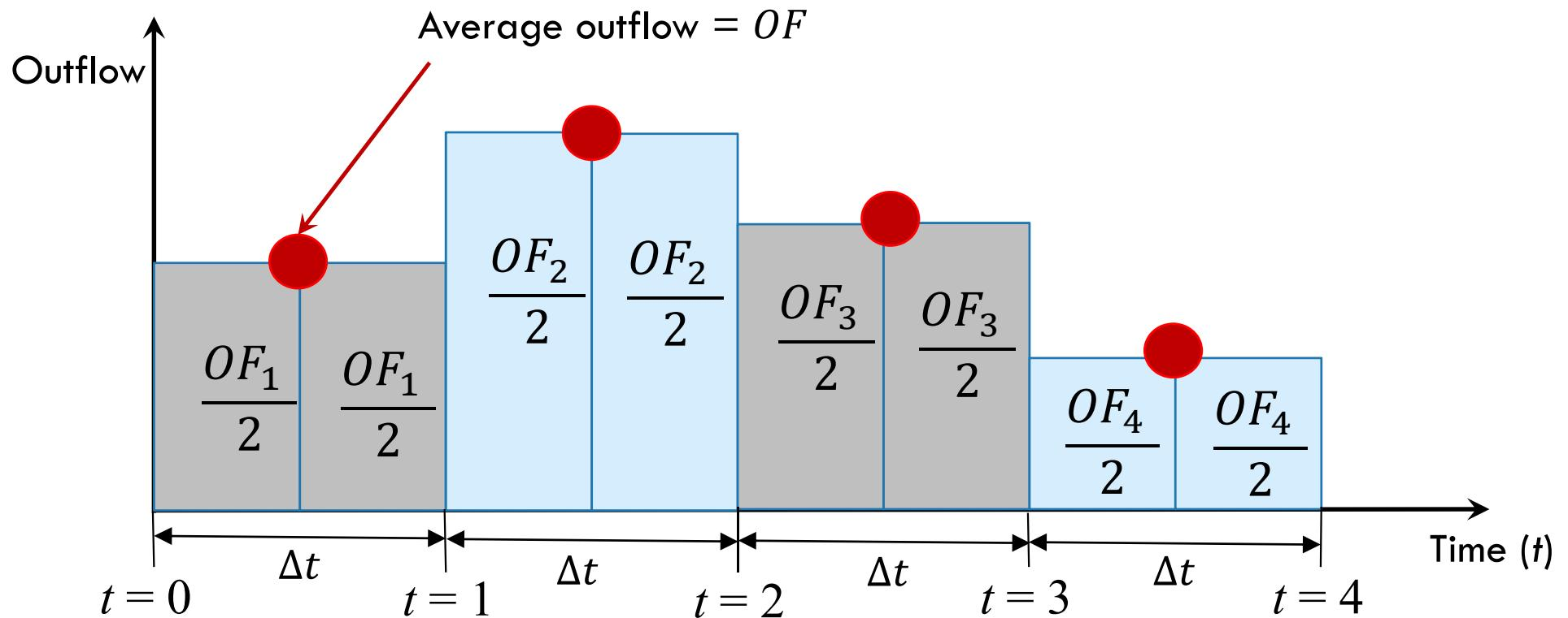
$$\Sigma I - \Sigma O = \frac{\Delta S}{\Delta t} \rightarrow S_{t+1} - S_t = (\Sigma I - \Sigma O) \Delta t$$
