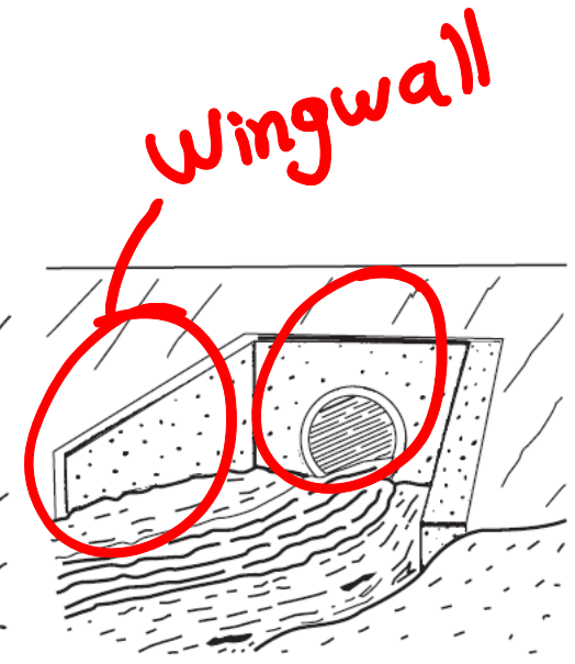
Cast-in-place concrete headwall and wingwalls
