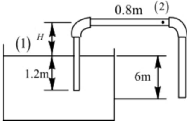
Energy Equation: Since point 1 and 3 are open to atmosphere and velocity at point 1 is zero, the energy equation reduces to:
