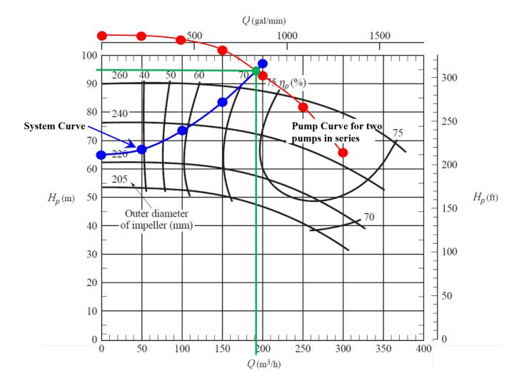
$$\begin{array}{l} (4) \\ D = 0.10 \text{ m, } L = 120 \text{ m, } f = 0.02, \quad \Sigma \text{ k} = 3.2 \\ Q =?, \quad H =?, \quad Z_2 - \mathbb{Z}_1 = 65 \text{ m} \\ \text{System curve} \\ \text{Hp} = Z_2 - \mathbb{Z}_1 + \left(\frac{fL}{D} + \Sigma \text{ k}\right) \frac{Q^2}{Q} \\ Hp = 65 + \left(\frac{0.02 \times 50}{0.10} + 3.2\right) \frac{Q^2}{19.6} \left(\frac{\pi \times 0.1^2}{4}\right)^2 \\ \text{Hp} = 65 + 10917.9 \quad Q^2 \\ Q \text{ is in } \frac{m^3/s}{2} \end{array}$$
