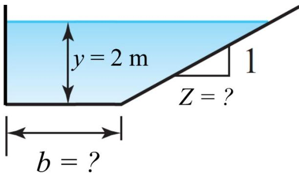
$$\textcircled{5} \quad Q = 10 \text{ m}^3/\text{s} \quad Q = A V$$
