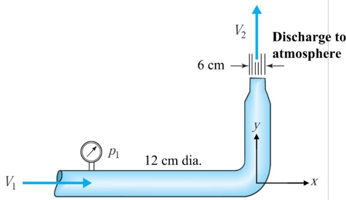
$$\sum F = \dot{m} (V_2 - V_1) \quad [\text{Momentum eq.}]$$
