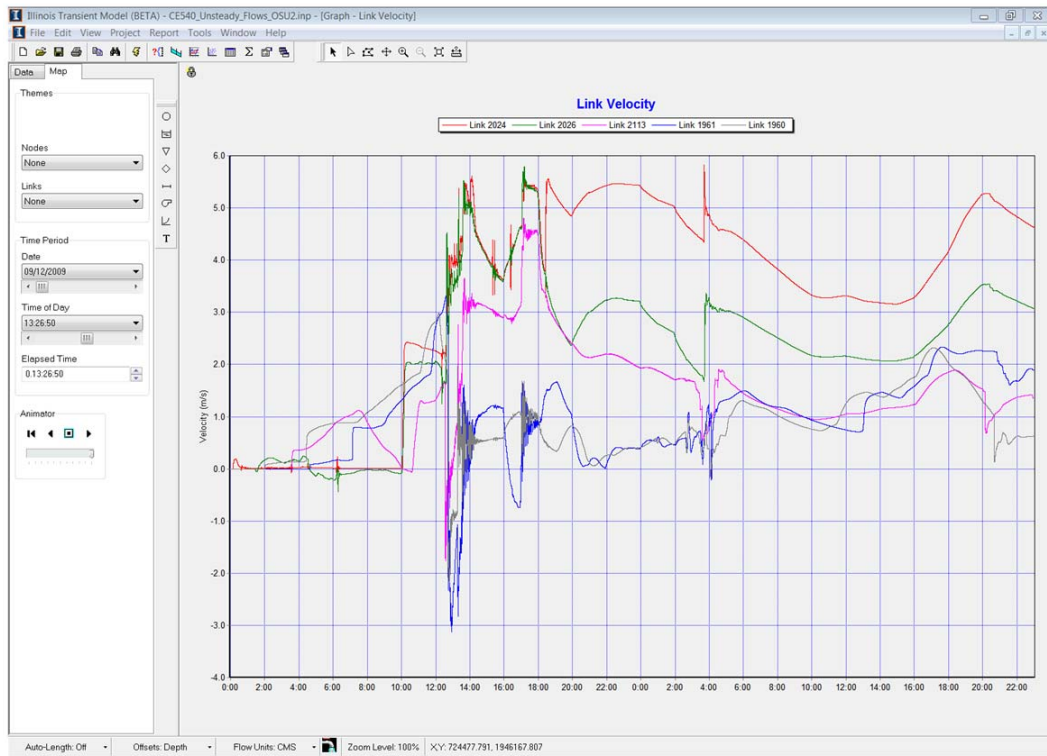
Figure 5.16: Flow velocity traces at the center of various tunnel reaches for the coarse output time (Initial dry bed state, a = 200 m/s).
