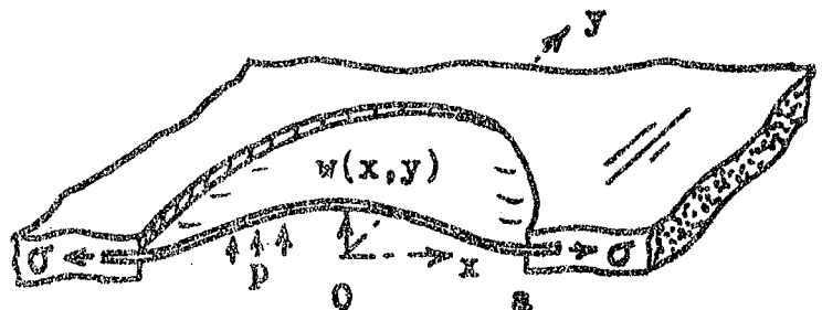
Fig. 4.4. Deflection due to pressure difference across slightly rigid membrane under tension
