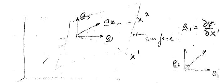
$\underline{q}_i$  are the unit vectors  $\underline{q}_1, \underline{q}_2$  are in surface.
