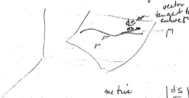
$$\text{metric} \quad \left| \frac{ds}{d\lambda} \right|^2 = \frac{dr}{d\lambda} \cdot \frac{dr}{d\lambda} = \underline{a}^\alpha \underline{a}^\beta \frac{dx^\alpha}{d\lambda} \frac{dx^\beta}{d\lambda}$$
