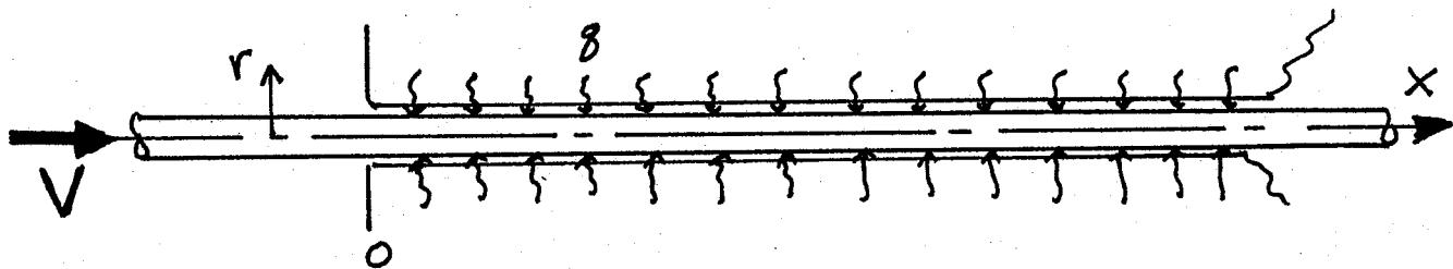
The equation describing the temperature field in the wire is\* (neglecting axial heat conduction)
