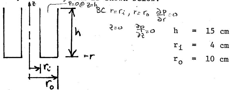
The equation governing the acoustic pressure field in the annular chamber is
