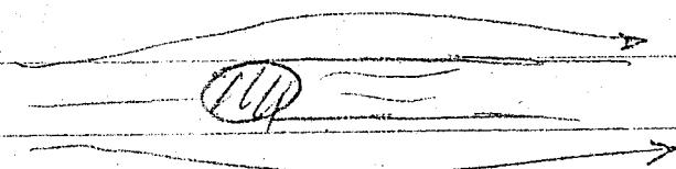
Laminar Separation of Boundary Layers
