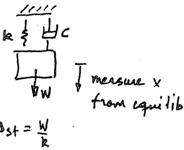
$F = c\dot{x}$  in direction opposite to motion  $[c] = \frac{\text{lb} \cdot \text{sec}}{\text{ft}} = \frac{\text{N} \cdot \text{s}}{\text{m}}$
