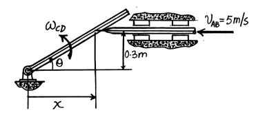
\***R2–20.** Determine the angular acceleration of rod *CD* at the instant  $\theta = 30^{\circ}$ . Rod *AB* has zero velocity, i.e.,  $v_{AB} = 0$ , and an acceleration of  $a_{AB} = 2 \text{ m/s}^2$  to the right when  $\theta = 30^{\circ}$ .
