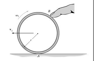
**Equations of Motion:** The mass moment of inertia of the ring about its mass center is given by  $I_G = mr^2$ . Applying Eq. 17–16, we have
