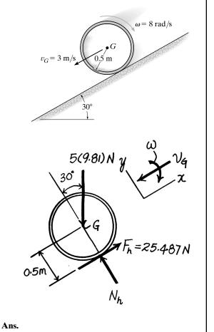
**R2–18.** The hoop (thin ring) has a mass of 5 kg and is released down the inclined plane such that it has a backspin  $\omega = 8 \text{ rad/s}$  and its center has a velocity  $v_G = 3 \text{ m/s}$  as shown. If the coefficient of kinetic friction between the hoop and the plane is  $\mu_k = 0.6$ , determine the hoop's angular velocity 1 s after it is released.
