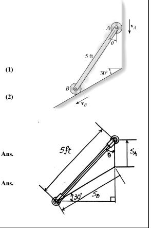
\***R2–36.** The bar is confined to move along the vertical and inclined planes. If the roller at *A* has a constant velocity of  $v_A = 6$  ft/s, determine the bar's angular acceleration and the acceleration of *B* when  $\theta = 45^{\circ}$ .
