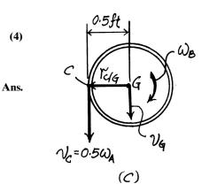
**R2-41.** A cord is wrapped around the rim of each 10-lb disk. If disk *B* is released from rest, determine how much time *t* is required before *A* attains an angular velocity  $\omega_A = 5$  rad/s.
