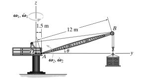
The xyz rotating frame is set parallel to the fixed XYZ frame with its origin attached to point A, Fig. a. Thus, the angular velocity and angular acceleration of this frame with respect to the XYZ frame are
