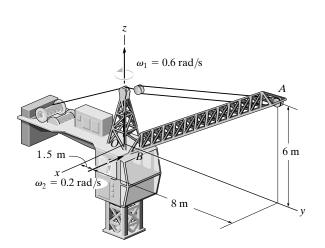
**Coordinate Axes:** The rotating *x*, *y*, *z* frame and fixed and fixed *X*, *Y*, *Z* frame are set with the origin at point *B* and *O* respectively.
