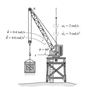
**Coordinate Axis:** The rotating *x*, *y*, *z* frame is set to be coincident with the fixed *X*, *Y*, *Z* frame with origin at point *B*.
