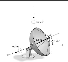
**Angular Velocity:** The coordinate axes for the fixed frame (X, Y, Z) and rotating frame (x, y, z) at the instant shown are set to be coincident. Thus, the angular velocity of the satellite at this instant (with reference to X, Y, Z) can be expressed in terms of **i**, **j**, **k** components.
