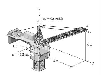
**Coordinate Axes:** The rotating *x*, *y*, *z* frame and fixed *X*, *Y*, *Z* frame are set with the origin at point *B* and *O* respectively.
