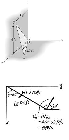
\*20-36. The triangular plate *ABC* is supported at *A* by a ball-and-socket joint and at *C* by the x-z plane. The side *AB* lies in the x-y plane. At the instant  $\theta = 60^{\circ}$ ,  $\dot{\theta} = 2 \text{ rad/s}$ ,  $\ddot{\theta} = 3 \text{ rad/s}^2$  and point *C* has the coordinates shown. Determine the angular acceleration of the plate and the acceleration of point *C* at this instant.
