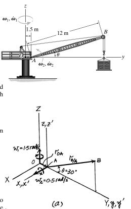
•20–53. At the instant  $\theta = 30^\circ$ , the frame of the crane is rotating with an angular velocity of  $\omega_1 = 1.5$  rad/s and angular acceleration of  $\dot{\omega}_1 = 0.5$  rad/s<sup>2</sup>, while the boom *AB* rotates with an angular velocity of  $\omega_2 = 0.5$  rad/s and angular acceleration of  $\dot{\omega}_2 = 0.25$  rad/s<sup>2</sup>. Determine the velocity and acceleration of point *B* at this instant.
