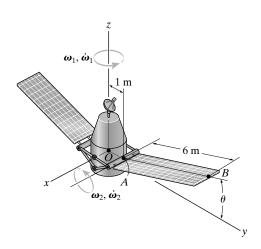
The xyz rotating frame is set parallel to the fixed XYZ frame with its origin attached to point A, Fig. a. Thus, the angular velocity and angular acceleration of this frame with respect to the XYZ frame are
