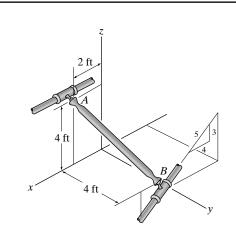
**20–26.** When rod *AB* is in the position shown, collar *A* moves with a velocity of  $\mathbf{v}_A = \{10\mathbf{i}\}$  ft/s and acceleration of  $\mathbf{a}_A = \{2\mathbf{i}\}$  ft/s<sup>2</sup>. Determine the acceleration of collar *B* at this instant. Assume the angular velocity and angular acceleration of *AB* are perpendicular to the rod.
