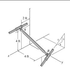
**20–27.** If collar *A* moves with a constant velocity of  $\mathbf{v}_A = \{3\mathbf{i}\}\ \mathbf{m/s}$ , determine the velocity of collar *B* when rod *AB* is in the position shown. Assume the angular velocity of *AB* is perpendicular to the rod.
