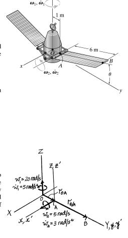
•20–17. At the instant  $\theta = 30^\circ$ , the satellite's body is rotating with an angular velocity of  $\omega_1 = 20$  rad/s, and it has an angular acceleration of  $\dot{\omega}_1 = 5$  rad/s<sup>2</sup>. Simultaneously, the solar panels rotate with a constant angular velocity of  $\omega_2 = 5$  rad/s. Determine the velocity and acceleration of point *B* located at the end of one of the solar panels at this instant.
