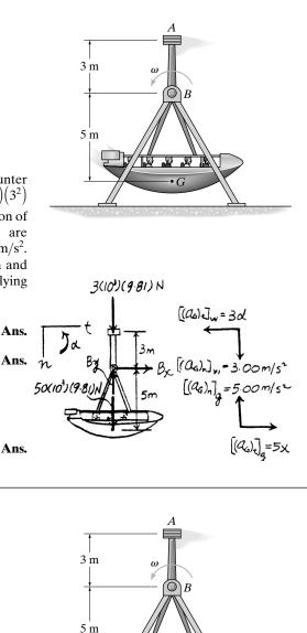
•17-65. The passengers, the gondola, and its swing frame have a total mass of 50 Mg, a mass center at G, and a radius of gyration  $k_B = 3.5$  m. Additionally, the 3-Mg steel block at A can be considered as a point of concentrated mass. Determine the angle  $\theta$  to which the gondola will swing before it stops momentarily, if it has an angular velocity of  $\omega = 1$  rad/s at its lowest point.
