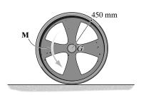
**Equations of Motion:** The mass moment of inertia of the wheel about its mass center is  $I_G = mk_G^2 = 75(0.375^2) = 10.55 \text{ kg} \cdot \text{m}^2$ . Writing the moment equation of motion about point A, we have
