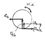
\*17–112. The assembly consists of an 8-kg disk and a 10-kg bar which is pin connected to the disk. If the system is released from rest, determine the angular acceleration of the disk. The coefficients of static and kinetic friction between the disk and the inclined plane are  $\mu_s = 0.6$  and  $\mu_k = 0.4$ , respectively. Neglect friction at *B*.
