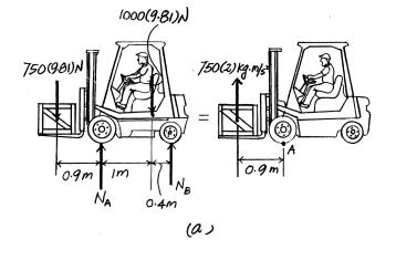
\*17–48. Determine the greatest acceleration with which the 1-Mg forklift can raise the 750-kg crate, without causing the wheels at *B* to leave the ground. The centers of mass for the forklift and the crate are located at  $G_1$  and  $G_2$ , respectively.
