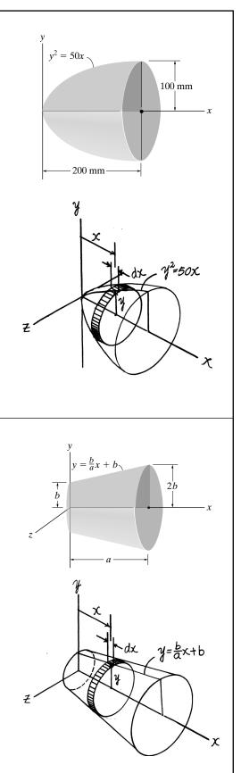
•17–5. The paraboloid is formed by revolving the shaded area around the x axis. Determine the moment of inertia about the x axis and express the result in terms of the total mass m of the paraboloid. The material has a constant density  $\rho$ .
