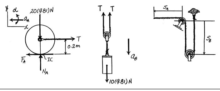
**17–115.** Determine the minimum coefficient of static friction between the disk and the surface in Prob. 17–114 so that the disk will roll without slipping. Neglect the mass of the pulleys.
