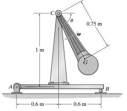
**17–79.** If the support at *B* is suddenly removed, determine the initial horizontal and vertical components of reaction that the pin *A* exerts on the rod *ACB*. Segments *AC* and *CB* each have a weight of 10 lb.
