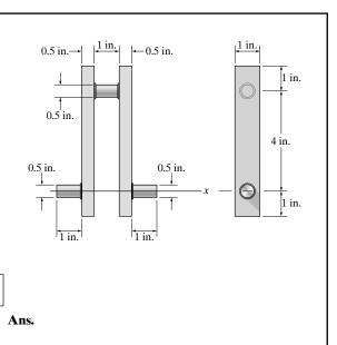
**17–19.** Determine the moment of inertia of the overhung crank about the x axis. The material is steel for which the density is  $\rho = 7.85 \text{ Mg/m}^3$ .
