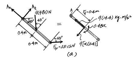
**17–75.** Determine the angular acceleration of the 25-kg diving board and the horizontal and vertical components of reaction at the pin A the instant the man jumps off. Assume that the board is uniform and rigid, and that at the instant he jumps off the spring is compressed a maximum amount of 200 mm,  $\omega = 0$ , and the board is horizontal. Take k = 7 kN/m.
