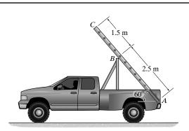
**Equations of Motion:** We must first show that the ladder will rotate when the acceleration of the truck is  $6 \text{ m/s}^2$ . This can be done by determining the minimum acceleration of the truck that will cause the ladder to lose contact at B,  $N_B = 0$ . Writing the moment equation of motion about point A using Fig. a,
