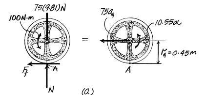
**17–122.** The 75-kg wheel has a radius of gyration about its mass center of  $k_G = 375$  mm. If it is subjected to a torque of  $M = 150 \text{ N} \cdot \text{m}$ , determine its angular acceleration. The coefficients of static and kinetic friction between the wheel and the ground are  $\mu_s = 0.2$  and  $\mu_k = 0.15$ , respectively.
