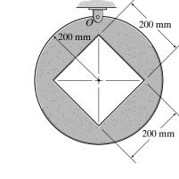
\*17–24. The 4-Mg uniform canister contains nuclear waste material encased in concrete. If the mass of the spreader beam *BD* is 50 kg, determine the force in each of the links *AB*, *CD*, *EF*, and *GH* when the system is lifted with an acceleration of  $a = 2 \text{ m/s}^2$  for a short period of time.
