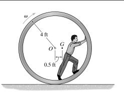
**Equations of Motion:** The mass moment of inertia of the system about its mass center is  $I_G = mk_G^2 = \frac{500}{32.2}(3.5^2) = 190.22$  slug  $\cdot$  ft<sup>2</sup>. Writing the moment equation of motion about point *A*, Fig. *a*,
