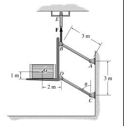
**17–55.** A uniform plate has a weight of 50 lb. Link *AB* is subjected to a couple moment of  $M = 10 \text{ lb} \cdot \text{ft}$  and has a clockwise angular velocity of 2 rad/s at the instant  $\theta = 30^{\circ}$ . Determine the force developed in link *CD* and the tangential component of the acceleration of the plate's mass center at this instant. Neglect the mass of links *AB* and *CD*.
