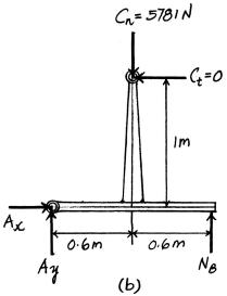
**17–78.** The 100-kg pendulum has a center of mass at G and a radius of gyration about G of  $k_G = 250$  mm. Determine the horizontal and vertical components of reaction on the beam by the pin A and the normal reaction of the roller B at the instant  $\theta = 0^\circ$  when the pendulum is rotating at  $\omega = 4$  rad/s. Neglect the weight of the beam and the support.
