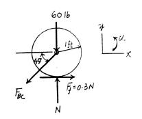
•17-89. A 17-kg roll of paper, originally at rest, is supported by bracket *AB*. If the roll rests against a wall where the coefficient of kinetic friction is  $\mu_C = 0.3$ , and a constant force of 30 N is applied to the end of the sheet, determine the tension in the bracket as the paper unwraps, and the angular acceleration of the roll. For the calculation, treat the roll as a cylinder.
