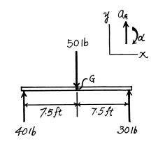
**Equations of Motion:** The mass moment of inertia of the plank about its mass center is given by  $I_G = \frac{1}{12} ml^2 = \frac{1}{12} \left(\frac{50}{32.2}\right) (15^2) = 29.115 \text{ slug} \cdot \text{ft}^2$  Applying Eq. 17–14, we have
