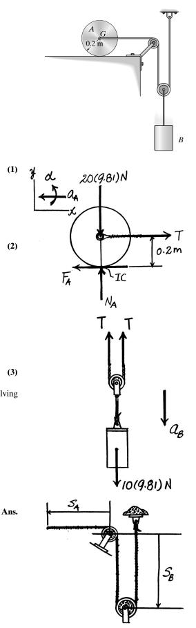
\*17-116. The 20-kg square plate is pinned to the 5-kg smooth collar. Determine the initial angular acceleration of the plate when P = 100 N is applied to the collar. The plate is originally at rest.
