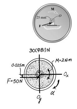
•17-61. If the motor in Prob. 17-60 is disengaged from the shaft once the flywheel is rotating at 15 rad/s, so that M = 0, determine how long it will take before the resultant bearing frictional force F = 50 N stops the flywheel from rotating.
