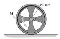
**Equations of Motion:** The mass moment of inertia of the wheel about its mass center is  $I_G = mk_G^2 = 75(0.375^2) = 10.55 \text{ kg} \cdot \text{m}^2$ . Writing the moment equation of motion about point A,
