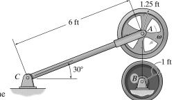
**Equations of Motion:** Since wheel *B* is fixed, wheel *A* will slip on wheel *B*. The frictional force developed at the contact point is  $F = \mu_k N = 0.3N$ . The mass moment
