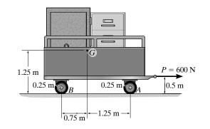
Equations of Motion: Writing the force equation of motion along the x axis,
