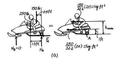
**17–50.** The snowmobile has a weight of 250 lb, centered at  $G_1$ , while the rider has a weight of 150 lb, centered at  $G_2$ . If h = 3 ft, determine the snowmobile's maximum permissible acceleration **a** so that its front skid does not lift off the ground. Also, find the traction (horizontal) force and the normal reaction under the rear tracks at A.
