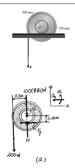
**17–119.** The spool has a mass of 100 kg and a radius of gyration of  $k_G = 200$  mm about its center of mass G. If a vertical force of P = 500 N is applied to the cable, determine the acceleration of G and the angular acceleration of the spool. The coefficients of static and kinetic friction between the rail and the spool are  $\mu_s = 0.2$  and  $\mu_k = 0.15$ , respectively.
