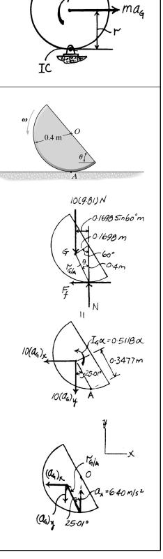
•17-93. The semicircular disk having a mass of 10 kg is rotating at  $\omega = 4$  rad/s at the instant  $\theta = 60^{\circ}$ . If the coefficient of static friction at A is  $\mu_s = 0.5$ , determine if the disk slips at this instant.
