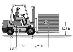
**Equations of Motion:** Since it is required that the rear wheels are about to leave the ground,  $N_A = 0$ . Applying the moment equation of motion of about point *B*,
