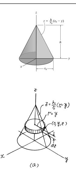
•17-9. Determine the mass moment of inertia  $I_y$  of the solid formed by revolving the shaded area around the y axis. The density of the material is  $\rho$ . Express the result in terms of the mass m of the solid.
