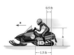
**Equations of Motion:** Since the front skid is required to be on the verge of lift off,  $N_B = 0$ . Writing the moment equation about point *A* and referring to Fig. *a*,
