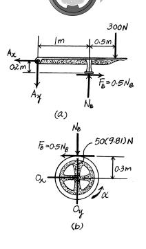
•17-85. The 50-kg flywheel has a radius of gyration about its center of mass of  $k_0 = 250$  mm. It rotates with a constant angular velocity of 1200 rev/min before the brake is applied. If the coefficient of kinetic friction between the brake pad Band the wheel's rim is  $\mu_k = 0.5$ , determine the constant force P that must be applied to the braking mechanism's handle in order to stop the wheel in 100 revolutions.
