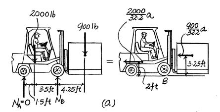
•17–37. If the forklift's rear wheels supply a combined traction force of  $F_A = 300$  lb, determine its acceleration and the normal reactions on the pairs of rear wheels and front wheels. The forklift has a weight of 2000 lb, with center of gravity at  $G_1$ , and the load weighs 900 lb, with center of gravity at  $G_2$ . The front wheels are free to roll. Neglect the weight of the wheels.
