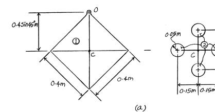
**17–23.** Determine the mass moment of inertia of the thin plate about an axis perpendicular to the page and passing through point O. The material has a mass per unit area of  $20 \text{ kg/m}^2$ .
