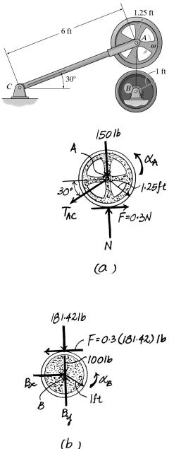
\*17–72. Initially, wheel A rotates clockwise with a constant angular velocity of  $\omega = 100 \text{ rad/s}$ . If A is brought into contact with B, which is held fixed, determine the number of revolutions before wheel A is brought to a stop. The coefficient of kinetic friction between the two wheels is  $\mu_k = 0.3$ , and the radius of gyration of A about its mass center is  $k_A = 1$  ft. Neglect the weight of link AC.
