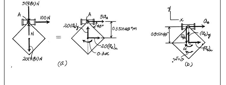
**17–118.** The spool has a mass of 100 kg and a radius of gyration of  $k_G = 200$  mm about its center of mass G. If a vertical force of P = 200 N is applied to the cable, determine the acceleration of G and the angular acceleration of the spool. The coefficients of static and kinetic friction between the rail and the spool are  $\mu_s = 0.3$  and  $\mu_k = 0.25$ , respectively.
