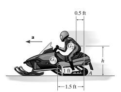
**Equations of Motion:** Since the front skid is required to be on the verge of lift off,  $N_B = 0$ . Writing the moment equation about point *A* and referring to Fig. *a*,
