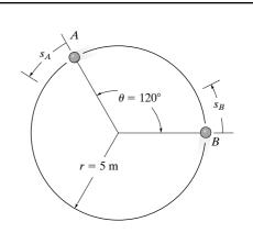
**12–151.** The race car travels around the circular track with a speed of 16 m/s. When it reaches point *A* it increases its speed at  $a_t = (\frac{4}{3}v^{1/4}) \text{ m/s}^2$ , where *v* is in m/s. Determine the magnitudes of the velocity and acceleration of the car when it reaches point *B*. Also, how much time is required for it to travel from *A* to *B*?
