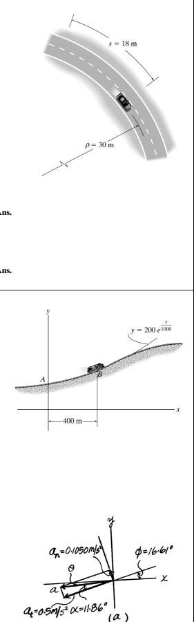
**12–122.** The train passes point A with a speed of 30 m/s and begins to decrease its speed at a constant rate of  $a_t = -0.25 \text{ m/s}^2$ . Determine the magnitude of the acceleration of the train when it reaches point B, where  $s_{AB} = 412 \text{ m}$ .
