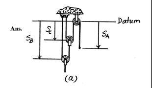
\*12–204. The crane is used to hoist the load. If the motors at A and B are drawing in the cable at a speed of 2 ft/s and 4 ft/s, respectively, determine the speed of the load.
