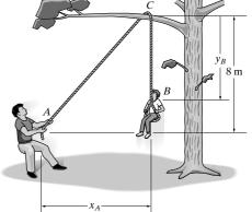
•12–213. The man pulls the boy up to the tree limb *C* by walking backward. If he starts from rest when  $x_A = 0$  and moves backward with a constant acceleration  $a_A = 0.2 \text{ m/s}^2$ , determine the speed of the boy at the instant  $y_B = 4 \text{ m}$ . Neglect the size of the limb. When  $x_A = 0$ ,  $y_B = 8 \text{ m}$ , so that *A* and *B* are coincident, i.e., the rope is 16 m long.
