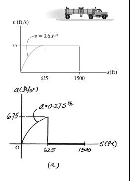
**12–51.** A car starts from rest and travels along a straight road with a velocity described by the graph. Determine the total distance traveled until the car stops. Construct the s-t and a-t graphs.
