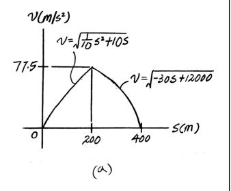
**12–58.** A sports car travels along a straight road with an acceleration-deceleration described by the graph. If the car starts from rest, determine the distance s' the car travels until it stops. Construct the v-s graph for  $0 \le s \le s'$ .
