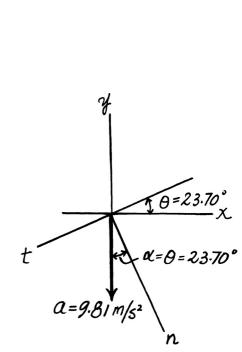
**12–154.** The motion of a particle is defined by the equations  $x = (2t + t^2)$  m and  $y = (t^2)$  m, where t is in seconds. Determine the normal and tangential components of the particle's velocity and acceleration when t = 2 s.
