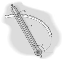
\*12–188. The partial surface of the cam is that of a logarithmic spiral  $r = (40e^{0.05\theta})$  mm, where  $\theta$  is in radians. If the cam rotates at a constant angular velocity of  $\dot{\theta} = 4$  rad/s, determine the magnitudes of the velocity and acceleration of the point on the cam that contacts the follower rod at the instant  $\theta = 30^{\circ}$ .
