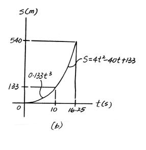
**12–70.** The a-t graph of the bullet train is shown. If the train starts from rest, determine the elapsed time t' before it again comes to rest. What is the total distance traveled during this time interval? Construct the v-t and s-t graphs.
