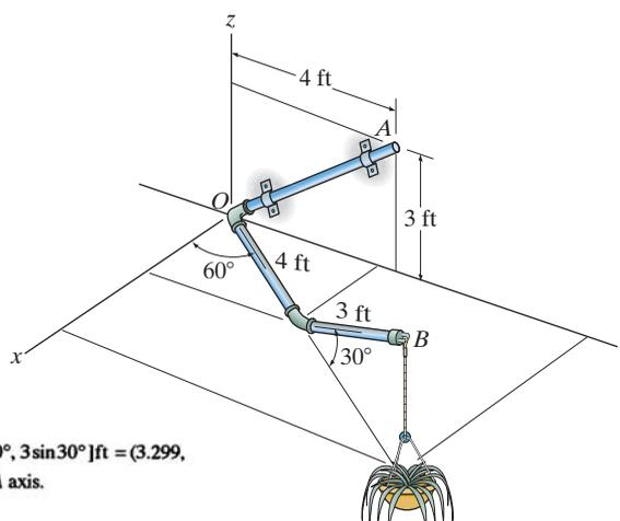
**Moment About the  $OA$  axis:** The coordinates of point  $B$  are  $[(4 + 3\cos 30^\circ)\cos 60^\circ, (4 + 3\cos 30^\circ)\sin 60^\circ, 3\sin 30^\circ]$  ft = (3.299, 5.714, 1.5) ft. Either position vector  $\mathbf{r}_{OB}$  or  $\mathbf{r}_{OC}$  can be used to determine the moment of  $\mathbf{W}$  about the  $OA$  axis.
