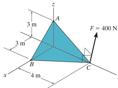
**Force Vector:** Since force  $\mathbf{F}$  is perpendicular to the inclined plane, its unit vector  $\mathbf{u}_F$  is equal to the unit vector of the cross product,  $\mathbf{b} = \mathbf{r}_{AC} \times \mathbf{r}_{BC}$ , Fig. *a*. Here
