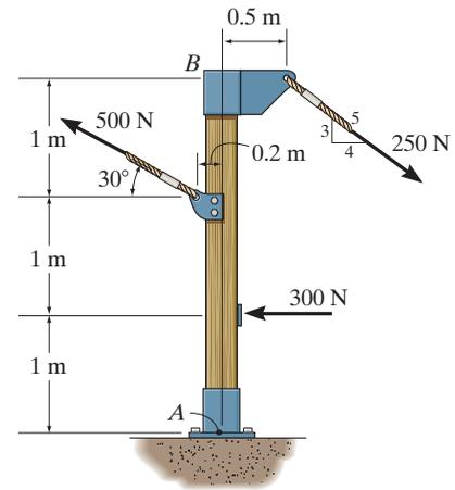
**Equivalent Resultant Force:** Forces  $F_1$  and  $F_2$  are resolved into their  $x$  and  $y$  components, Fig.  $a$ . Summing these force components algebraically along the  $x$  and  $y$  axes,
