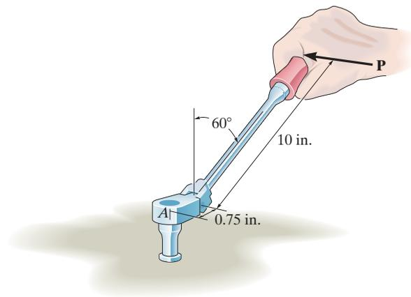
**4-67.** If a torque or moment of  $80 \text{ lb}\cdot\text{in.}$  is required to loosen the bolt at  $A$ , determine the force  $P$  that must be applied perpendicular to the handle of the flex-headed ratchet wrench.
