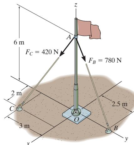
**Position Vector and Force Vectors:** Either position vector  $\mathbf{r}_{OA}$  or  $\mathbf{r}_{OB}$  can be used to determine the moment of  $\mathbf{F}_B$  about point  $O$ .
