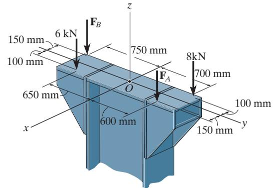
**Equivalent Resultant Force:** By equating the sum of the forces in Fig. *a* along the  $z$  axis to the resultant force  $F_R$ , Fig. *b*,
