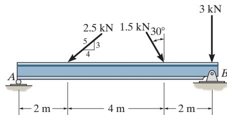
$$\begin{aligned} \rightarrow F_{R_x} = \Sigma F_x; \quad F_{R_x} &= 1.5 \sin 30^\circ - 2.5 \left(\frac{4}{5}\right) \\ &= -1.25 \text{ kN} = 1.25 \text{ kN} \leftarrow \end{aligned}$$
