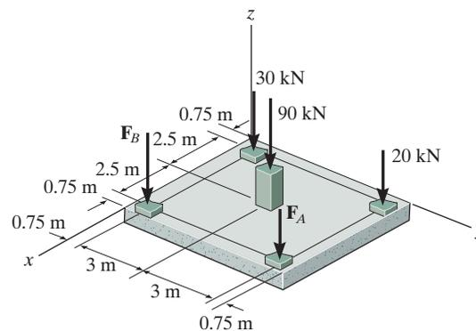
**Equivalent Resultant Force:** By equating the sum of the forces along the  $z$  axis to the resultant force  $F_R$ ,  $F_R \hat{=}$   $\hat{b}$ ,
