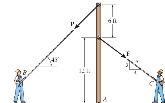
\*4-5. If the man at *B* exerts a force of  $P = 30$  lb on his rope, determine the magnitude of the force **F** the man at *C* must exert to prevent the pole from rotating, i.e., so the resultant moment about *A* of both forces is zero.
