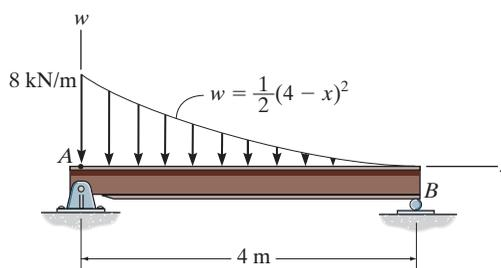
**Resultant:** The magnitude of the differential force  $dF_R$  is equal to the area of the element shown shaded in Fig. a. Thus,
