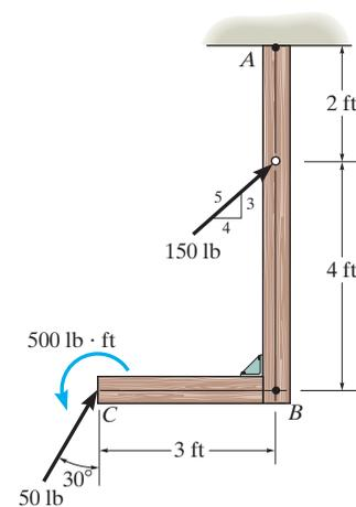
$$\rightarrow F_{Rx} = \Sigma F_x; \quad F_{Rx} = 150 \left(\frac{4}{5}\right) + 50 \sin 30^\circ = 145 \text{ lb}$$
