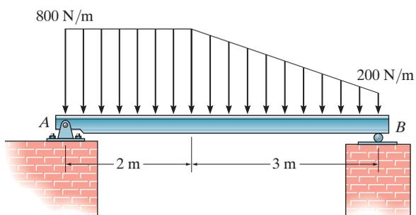
•4-145. Replace the distributed loading with an equivalent resultant force, and specify its location on the beam measured from point A.
