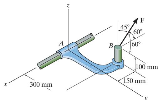
**Moment About the  $x$  axis:** The position vector  $\mathbf{r}_{AB}$ , Fig.  $a$ , will be used to determine the moment of  $\mathbf{F}$  about the  $x$  axis.
