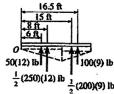
4-147. Determine the intensities  $w_1$  and  $w_2$  of the distributed loading acting on the bottom of the slab so that this loading has an equivalent resultant force that is equal but opposite to the resultant of the distributed loading acting on the top of the plate.
