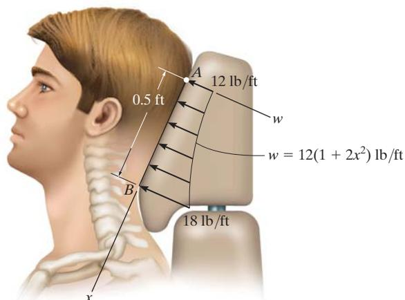
$$F_R = \int w(x) dx = \int_0^{0.5} 12(1 + 2x^2) dx = 12 \left[ x + \frac{2}{3}x^3 \right]_0^{0.5} = 7 \text{ lb} \quad \text{Ans}$$
