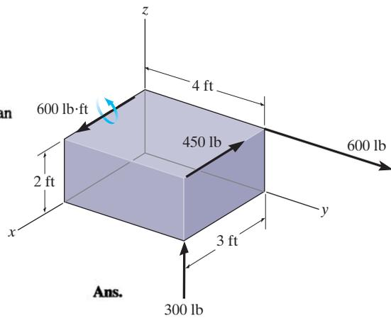
**Equivalent Couple Moment:** Here, we will assume that the axis of the wrench passes through point  $P$ , Figs.  $a$  and  $b$ . Since  $\mathbf{M}_W$  is collinear with  $\mathbf{F}_R$ ,
