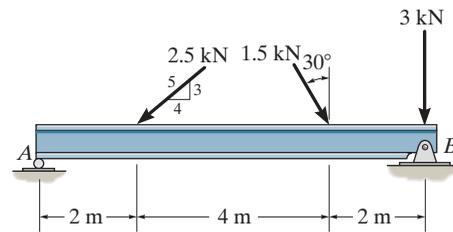
$$\begin{aligned} \rightarrow F_{R_x} = \Sigma F_x; \quad F_{R_x} &= 1.5 \sin 30^\circ - 2.5 \left(\frac{4}{5}\right) \\ &= -1.25 \text{ kN} = 1.25 \text{ kN} \leftarrow \end{aligned}$$
