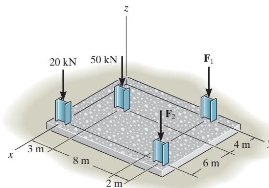
$$+\uparrow F_R = \Sigma F_z; \quad F_R = -20 - 50 - 30 - 40 = -140 \text{ kN} = 140 \text{ kN} \downarrow \quad \text{Ans}$$
