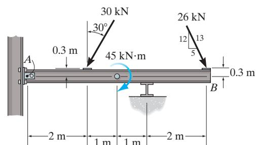
**Equivalent Resultant Force:** Forces  $F_1$  and  $F_2$  are resolved into their  $x$  and  $y$  components, Fig.  $a$ . Summing these force components algebraically along the  $x$  and  $y$  axes,
