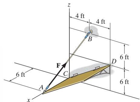
**Moment About the CD axis:** Either position vector  $\mathbf{r}_{CA}$  or  $\mathbf{r}_{CB}$ , Fig.  $a$ , can be used to determine the moment of  $F$  about the  $CD$  axis.
