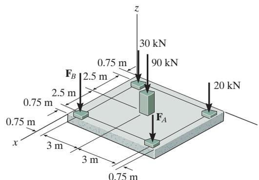
**Equivalent Resultant Force:** By equating the sum of the forces along the  $z$  axis to the resultant force  $F_R$ ,
