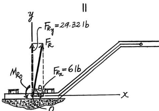
$$\rightarrow F_{Rx} = \Sigma F_x; \quad F_{Rx} = \frac{4}{5}(20) - 20 \sin 30^\circ = 6 \text{ lb}$$
