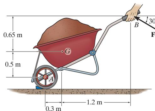
Resolving force  $F$  into its horizontal and vertical components, Fig.  $a$ , and applying the principle of moments,
