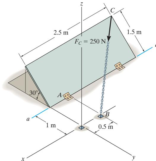
**\*4-168.** Determine the magnitude of the moment of the force  $F_C$  about the hinged axis  $aa$  of the door.
