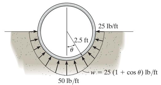
**Resultant Components:** The magnitude of the differential force  $dF_R$  is equal to the area of the element shown shaded in Fig. *a*.
