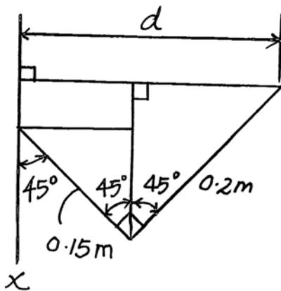
**Scalar Analysis:** From the geometry, the perpendicular distance from  $x$  axis to force  $\mathbf{F}$  is  $d = 0.15 \sin 45^\circ + 0.2 \sin 45^\circ = 0.2475 \text{ m}$ .
