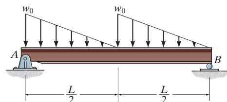
**Loading:** The distributed loading can be divided into two parts as shown in Fig. a. The magnitude and location of the resultant force of each part acting on the beam are also shown in Fig. a.
