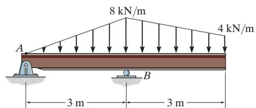
**Loading:** The distributed loading can be divided into three parts as shown in Fig. a.
