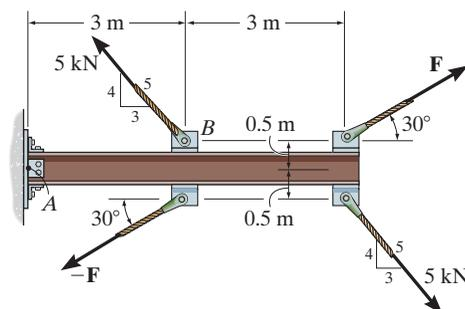
By resolving  $F$  and the 5 - kN couple into their  $x$  and  $y$  components, Fig.  $a$ , the couple moments  $(M_c)_1$  and  $(M_c)_2$  produced by  $F$  and the 5 - kN couple, respectively, are given by
