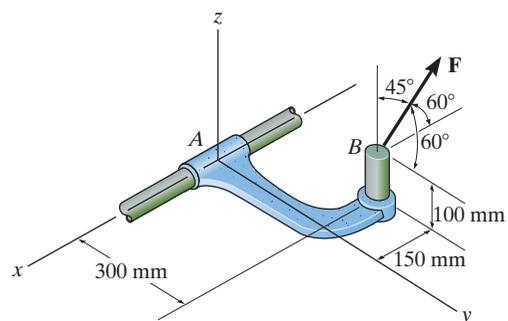
**Moment About the  $x$  axis:** Either position vector  $\mathbf{r}_{AB}$  or  $\mathbf{r}_{CB}$  can be used to determine the moment of  $\mathbf{F}$  about the  $x$  axis.
