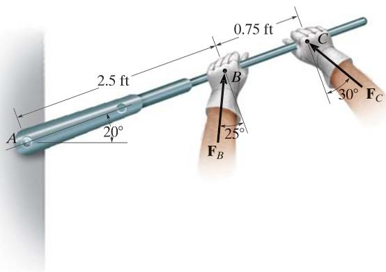
4-31. The rod on the power control mechanism for a business jet is subjected to a force of 80 N. Determine the moment of this force about the bearing at  $A$ .
