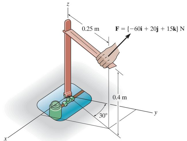
4-54. Determine the magnitude of the moments of the force  $\mathbf{F}$  about the  $x$ ,  $y$ , and  $z$  axes. Solve the problem (a) using a Cartesian vector approach and (b) using a scalar approach.
