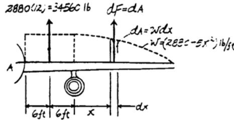
4-158. The distributed load acts on the beam as shown. Determine the magnitude of the equivalent resultant force and specify where it acts, measured from point  $A$ .
