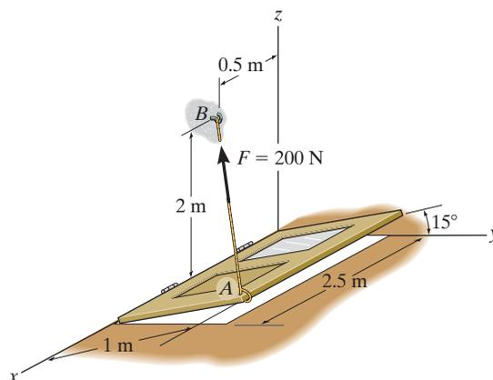
**Moment About the x axis:** Either position vector  $r_{OB}$  or  $r_{CA}$  can be used to determine the moment of  $F$  about the  $x$  axis.
