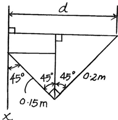
**Scalar Analysis :** From the geometry, the perpendicular distance from  $x$  axis to  $F$  is  $d = 0.15\sin 45^\circ + 0.2\sin 45^\circ = 0.2475$  m.
