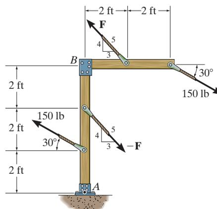
By resolving  $F$  and the  $150 \text{ lb}$  couple into their  $x$  and  $y$  components, Fig. a, the couple moments  $(M_C)_1$  and  $(M_C)_2$  produced by  $F$  and the  $5 \text{ kN}$  couple, respectively, are given by
