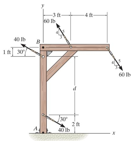
•4-89. Two couples act on the frame. If  $d = 4$  ft, determine the resultant couple moment. Compute the result by resolving each force into  $x$  and  $y$  components and (a) finding the moment of each couple (Eq. 4-13) and (b) summing the moments of all the force components about point  $A$ .
