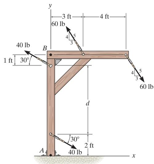
4-90. Two couples act on the frame. If  $d = 4$  ft, determine the resultant couple moment. Compute the result by resolving each force into  $x$  and  $y$  components and (a) finding the moment of each couple (Eq. 4-13) and (b) summing the moments of all the force components about point  $B$ .
