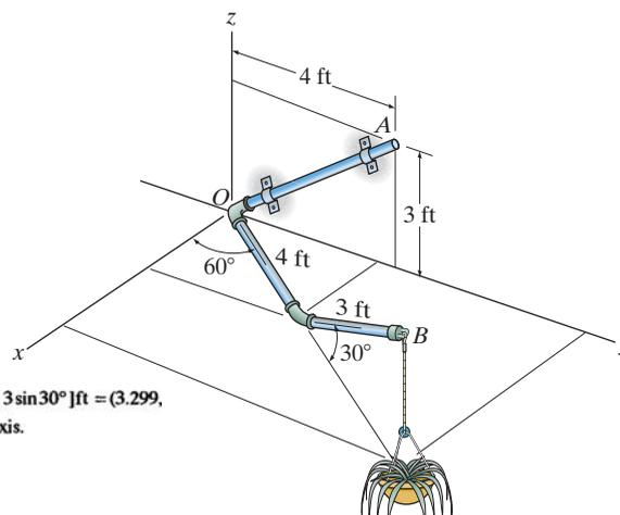
**Moment About the  $OA$  axis:** The coordinates of point  $B$  are  $[(4 + 3\cos 30^\circ)\cos 60^\circ, (4 + 3\cos 30^\circ)\sin 60^\circ, 3\sin 30^\circ]$  ft = (3.299, 5.714, 1.5) ft. Either position vector  $\mathbf{r}_{OB}$  or  $\mathbf{r}_{AB}$  can be used to determine the moment of  $\mathbf{W}$  about the  $OA$  axis.
