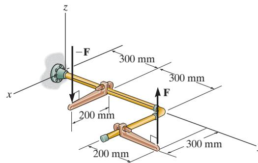
It is easiest to find the couple moment of  $\mathbf{F}$  by taking the moment of either  $\mathbf{F}$  or  $-\mathbf{F}$  about point  $A$  or  $B$ , respectively, Fig. *a*. Here the position vectors  $\mathbf{r}_{AB}$  and  $\mathbf{r}_{BA}$  must be determined first.
