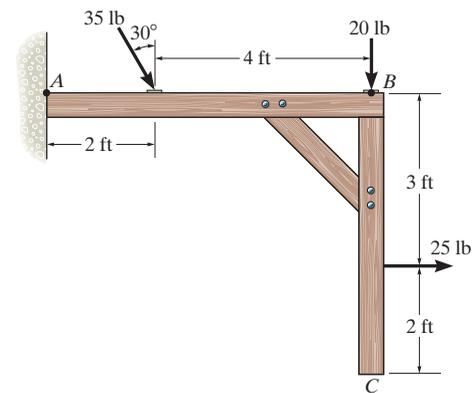
$$\rightarrow F_{R_x} = \Sigma F_x; \quad F_{R_x} = 35 \sin 30^\circ + 25 = 42.5 \text{ lb}$$
