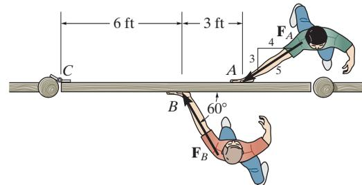
4-18. Two boys push on the gate as shown. If the boy at  $B$  exerts a force of  $F_B = 30$  lb, determine the magnitude of the force  $F_A$  the boy at  $A$  must exert in order to prevent the gate from turning. Neglect the thickness of the gate.
