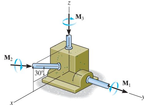
Since the couple moment is a free vector, it can act at any point without altering its effect. Thus, the couple moments  $M_1$ ,  $M_2$ , and  $M_3$  acting on the gear deducer can be simplified, as shown in Fig. a.
