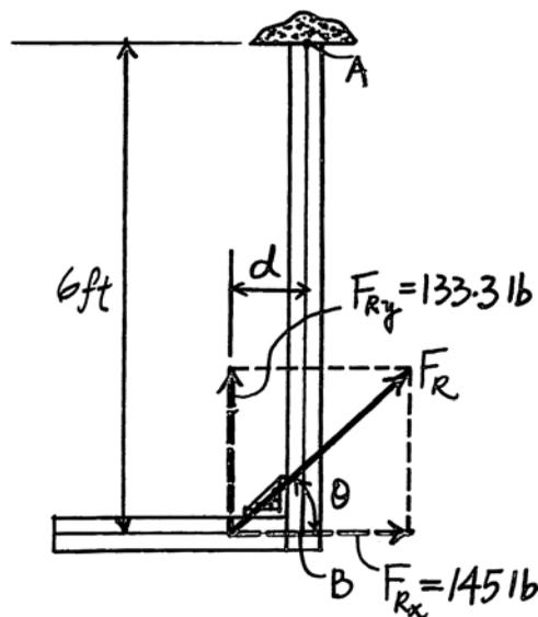
$$\rightarrow F_{Rx} = \Sigma F_x : F_{Rx} = 150 \left( \frac{4}{5} \right) + 50 \sin 30^\circ = 145 \text{ lb}$$
