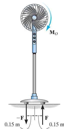
**Couple Moment:** The couple moment of  $F$  produces a counterclockwise moment of  $M_C = F(0.15 + 0.15) = 0.3F$ . Since the resultant couple moment about the axis perpendicular to the page is required to be zero,
