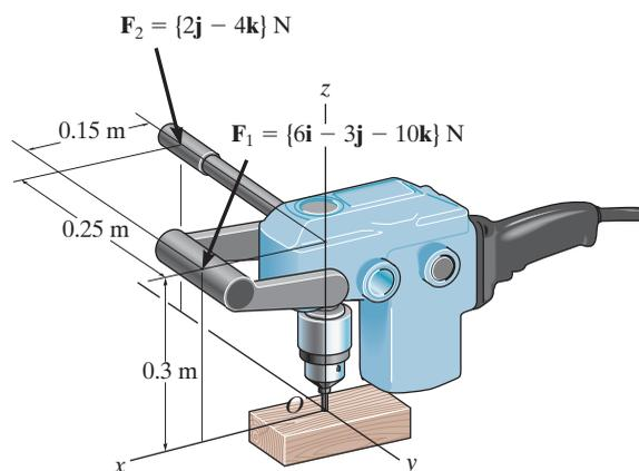
Note that  $F_{Rz} = -14 \text{ N}$  pushes the drill bit down into the stock.
