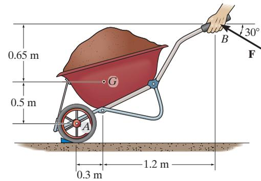
Resolving force  $\mathbf{F}$  into its horizontal and vertical components, Fig.  $a$ , and applying the principle of moments,
