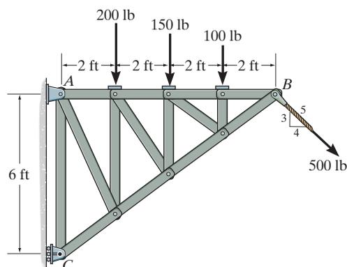
**Equivalent Resultant Force:** The 500-lb force is resolved into its  $x$  and  $y$  components, Fig. *a*. Summing these force components algebraically along the  $x$  and  $y$  axes,
