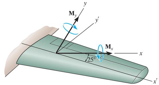
$$(M_R)_{x'} = \Sigma M_{x'}; \quad (M_R)_{x'} = 17 \cos 25^\circ - 25 \sin 25^\circ = 4.84 \text{ kip} \cdot \text{ft} \quad \text{Ans}$$
