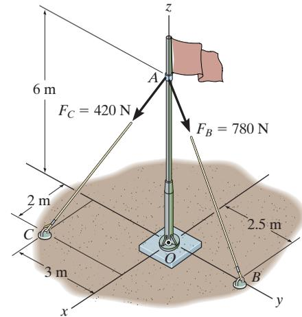
**Position Vector and Force Vectors:** The position vector  $r_{OA}$  and force vectors  $F_B$  and  $F_C$ , Fig. a, must be determined first.
