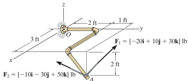
**Position Vector:** The position vector  $\mathbf{r}_{OA}$ , Fig.  $a$ , must be determined first.
