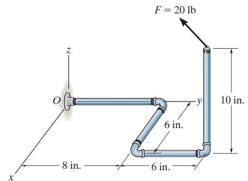
\*4-165. Determine the moment of the force  $\mathbf{F}$  about point  $O$ . The force has coordinate direction angles of  $\alpha = 60^\circ$ ,  $\beta = 120^\circ$ ,  $\gamma = 45^\circ$ . Express the result as a Cartesian vector.
