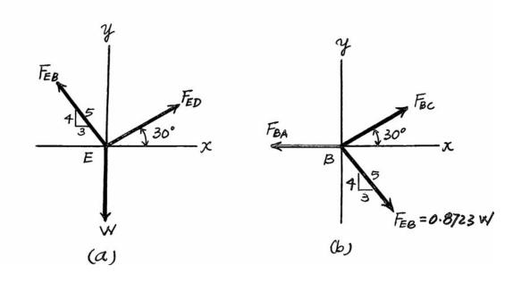
**3–26.** Determine the tensions developed in wires *CD*, *CB*, and BA and the angle  $\theta$  required for equilibrium of the 30-lb cylinder E and the 60-lb cylinder F.
