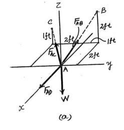
**3–50.** Determine the force in each cable needed to support the 3500-lb platform. Set d = 2 ft.
