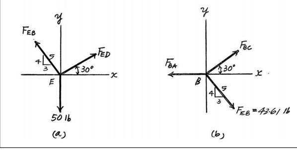
•3–25. Determine the maximum weight of the bucket that the wire system can support so that no single wire develops a tension exceeding 100 lb.
