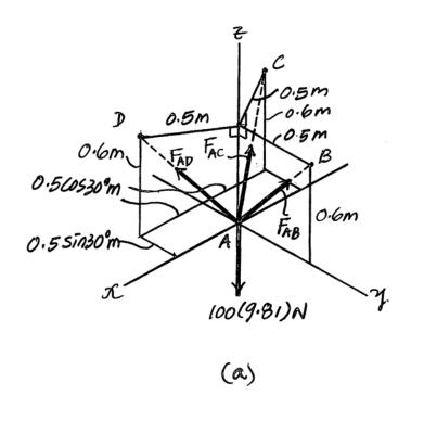
•3-65. The thin ring can be adjusted vertically between three equally long cables from which the 100-kg chandelier is suspended. If the ring remains in the horizontal plane and the tension in each cable is not allowed to exceed 1 kN, determine the smallest allowable distance z required for equilibrium.
