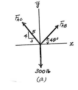
•3–9. If members AC and AB can support a maximum tension of 300 lb and 250 lb, respectively, determine the largest weight of the crate that can be safely supported.
