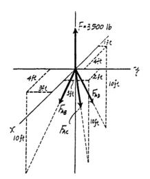
**3–51.** Determine the force in each cable needed to support the 3500-lb platform. Set d = 4 ft.
