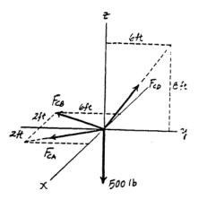
**3-79.** The joint of a space frame is subjected to four member forces. Member *OA* lies in the x-y plane and member *OB* lies in the y-z plane. Determine the forces acting in each of the members required for equilibrium of the joint.
