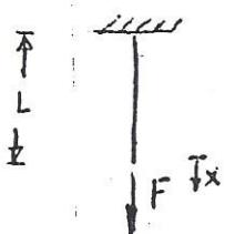
$$\sigma = F/A \quad \epsilon = \frac{\sigma}{E} = \frac{F}{AE} = \frac{x}{L} \quad U_c = \frac{\sigma^2}{2E} \cdot AL \quad U_s = \frac{F\epsilon^2}{2} \cdot AL$$
