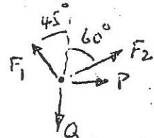
$$\begin{aligned} Q &= F_2 \cos 60^\circ + F_1 \cos 45^\circ \\ P &= F_1 \sin 45^\circ - F_2 \sin 60^\circ \end{aligned} \quad \left. \begin{array}{l} F_1 = \frac{\sqrt{3}-1}{\sqrt{2}} (P + \sqrt{3}Q) \\ F_2 = (\sqrt{3}-1)(Q-P) \end{array} \right\}$$
