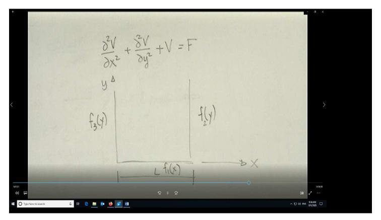
In this semi-infinite problem, at  $y=\infty$  the solution BC is that it must remain bounded. On the x=constant, the BCs can at most be functions of y, since x is fixed. On the y=constant line the BC can be at most a function of x.
