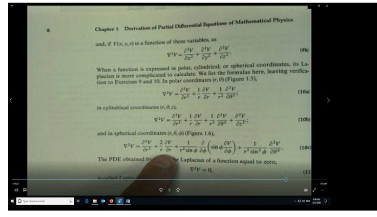
Here we show the definition of the Laplacian in different coordinate systems, Cartesian, cylindrical and spherical.
