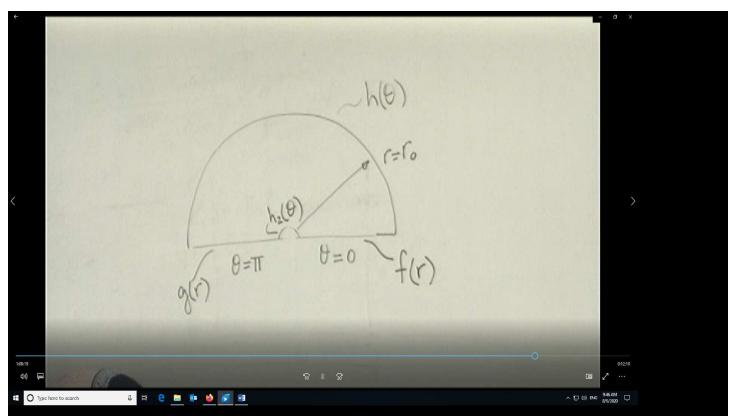
In the above, for  $\theta$ =constant lines, the BCs can be at most functions of r; similarly, on constant r lines, the BCs can be at most functions of theta.
