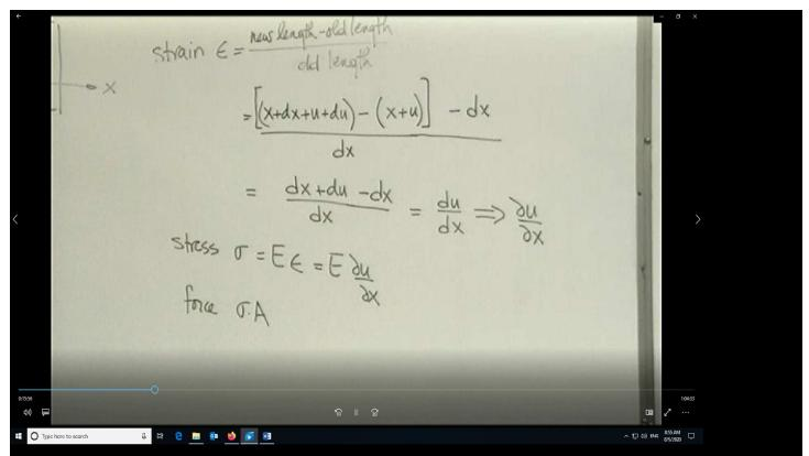
Force at any cross-section is  $\sigma \bullet A$  (A the cross-sectional area)=P. In 1-D we assume stress is the average across the cross-section.
