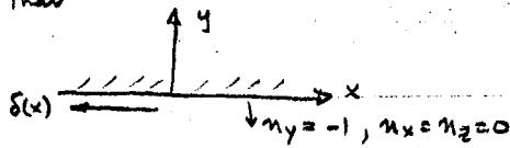
$$\therefore T_y = \sigma_{yy} n_j = -\sigma_{yy} = 0 \quad T_x = -\delta(x) = n_y \sigma_{xy} = -\sigma_{xy} \quad \text{thus } \sigma_{xy} \text{ must be to the left.}$$
