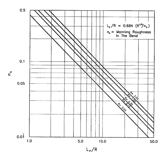
Protection Length, Lp, Downstream Of Channel Bend (11)
