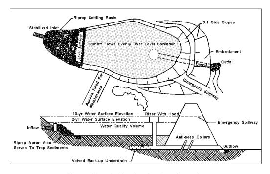
Figure 10-4. Infiltration basin schematic.
