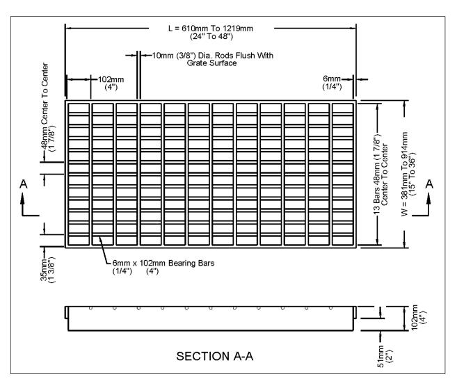
Figure 4-5. P-50 and P-50 x 100 grate (P-50 is this grate without 10mm (3/8") transverse rods).
