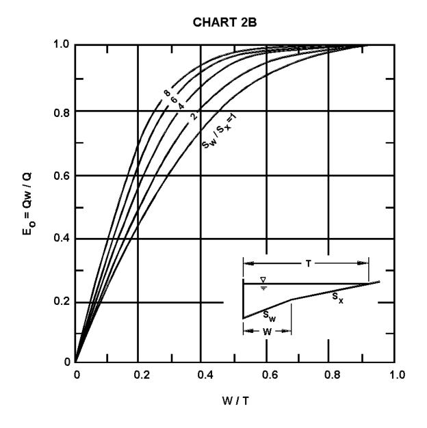
Ratio of Frontal Flow to Total Gutter Flow
