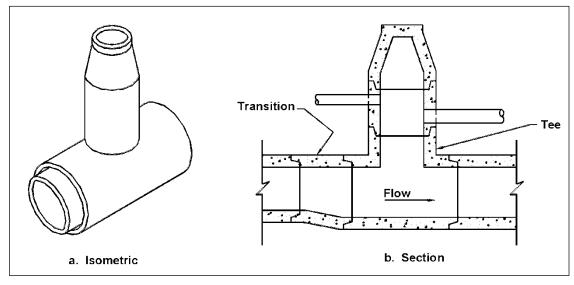
Figure 6-3. "Tee" access hole for large storm drains.
