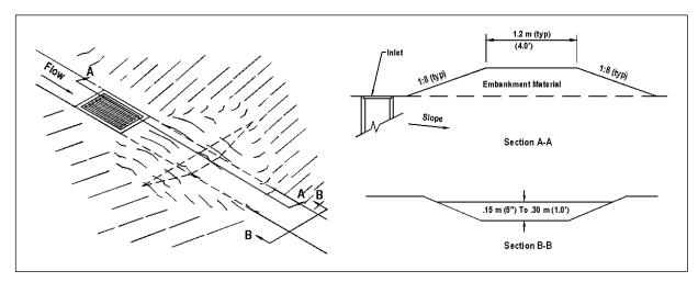
Figure 4-23. Median drop inlet. (85)
