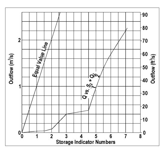
Figure 8-21. Storage indicator curve.
