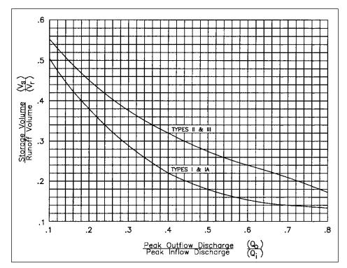
Figure 8-5. SCS detention basin routing curves. (13)
