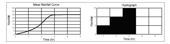
Figure 3-2. Example mass rainfall curve and corresponding hyetograph.
