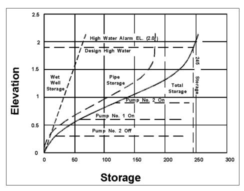
Figure 9-7. Stage-storage curve.
