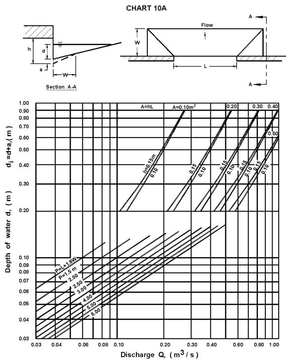
Depressed Curb-opening Inlet Capacity in Sump Locations
