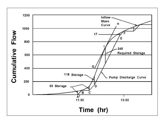
Figure 9-9. Mass curve routing diagram.
