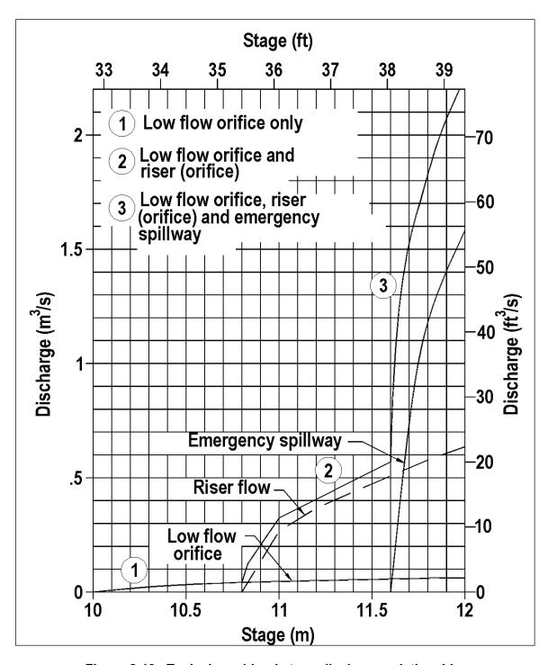
Figure 8-19. Typical combined stage-discharge relationship.
