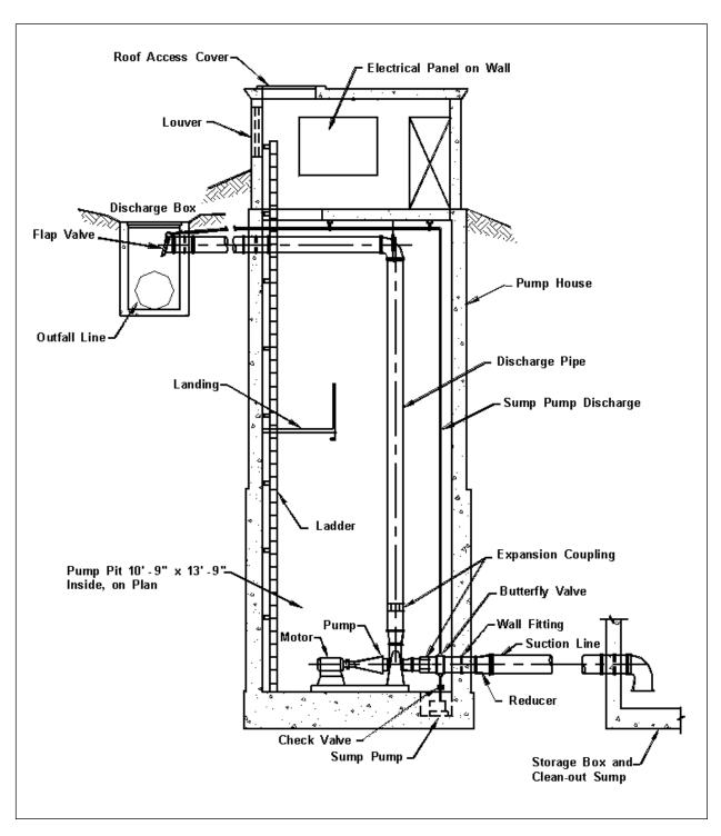
Figure 9-2. Typical dry-pit station. (51)
