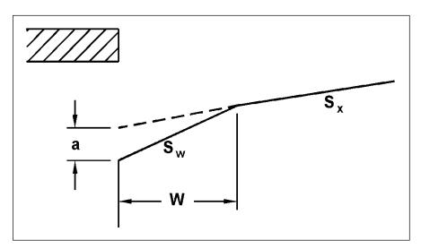
Figure 4-13. Depressed curb opening inlet.
