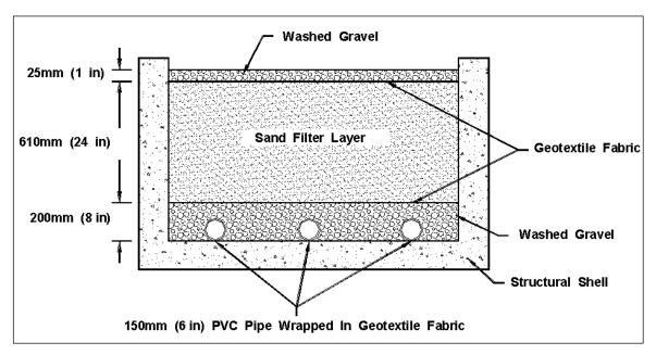
Figure 10-5. Cross-section schematic of sand filter compartment.
