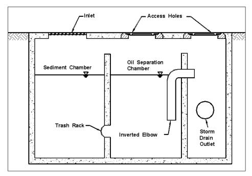
Figure 10-7. Cross-section detail of a typical oil/grit separator.
