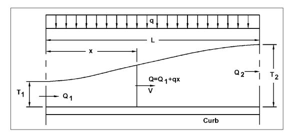
Figure B-1. Conceptual sketch of spatially varied gutter flow.
