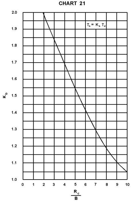
K<sub>b</sub> Factor For Maximum Shear Stress On Channel Bends. (12)
