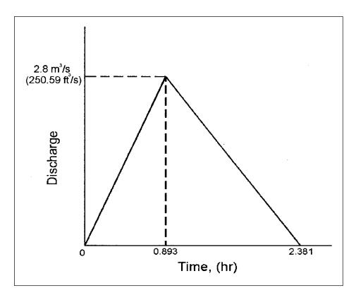
Figure 3-8. Example: The triangular unit hydrograph.
