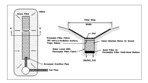
Figure 10-3. Median strip trench design.
