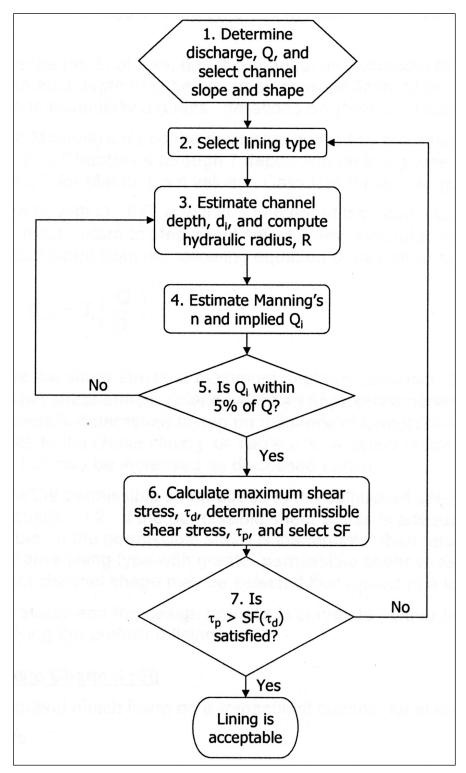
Figure 5-7. Flexible channel lining design flow chart (from HEC-15<sup>(34)</sup>).
