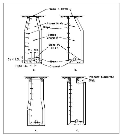
Figure 6-2. Typical access hole configurations.
