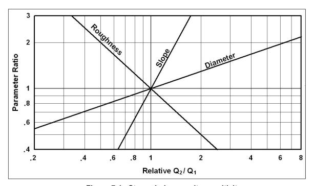
Figure 7-1. Storm drain capacity sensitivity.
