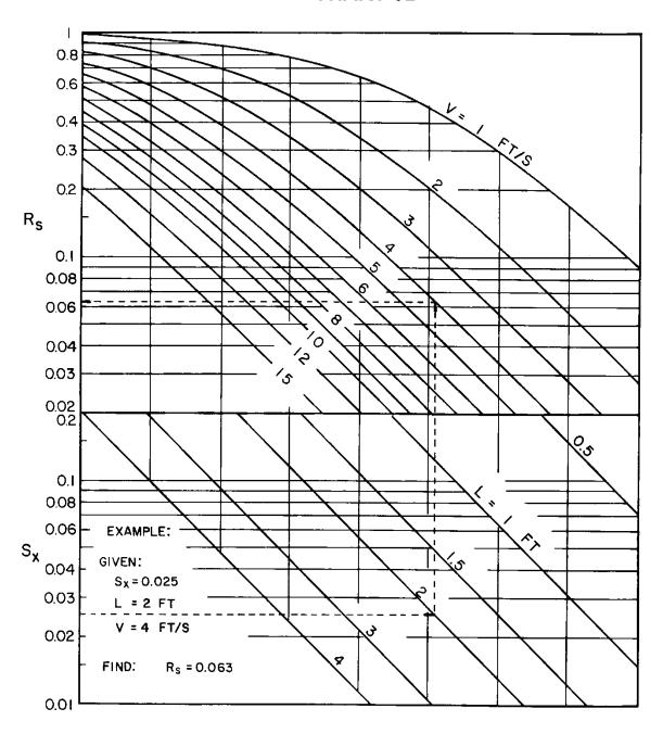
Grate Inlet Side Flow Intercept Efficiency
