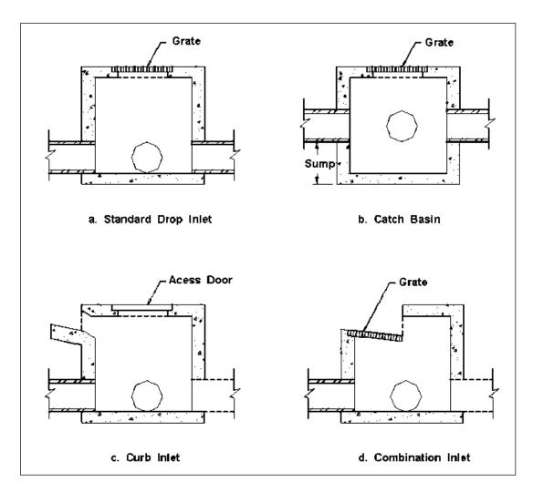
Figure 6-1. Inlet structures.
