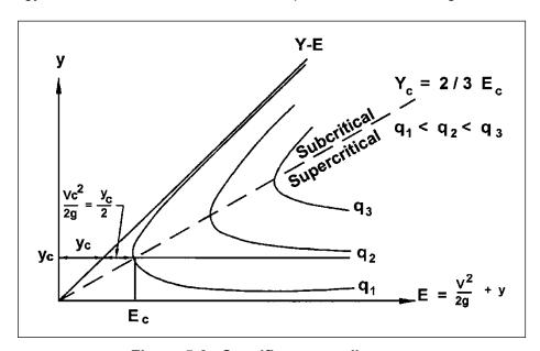
Figure 5-2. Specific energy diagram.
