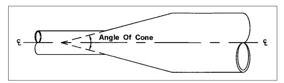
Figure 7-3. Angle of cone for pipe diameter changes.
