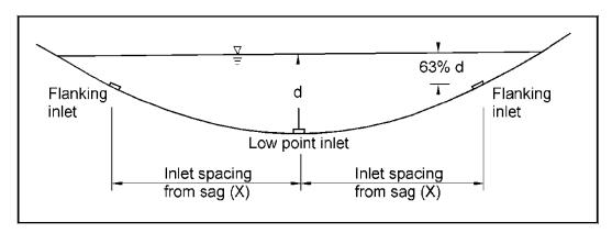
Figure 4-22. Example of flanking inlets.
