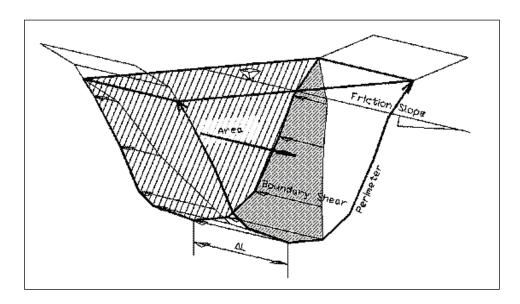
Figure 5-4. Distribution of shear stress.
