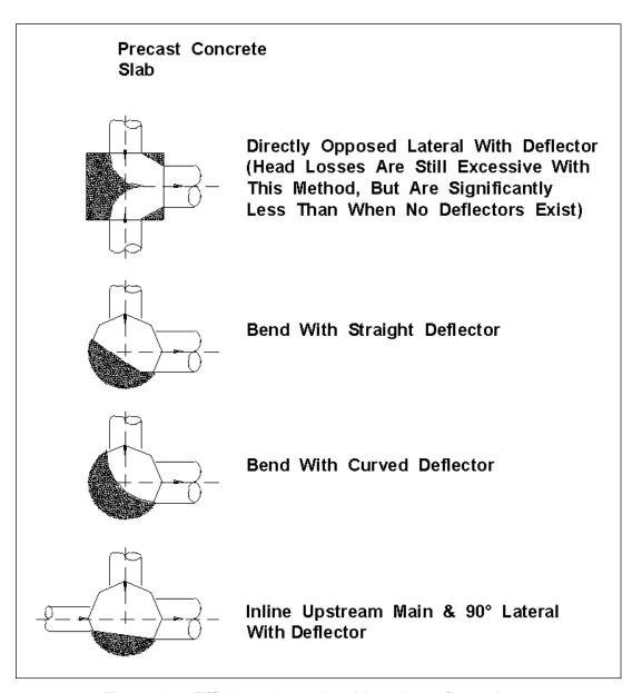
Figure 6-4. Efficient channel and bench configurations.
