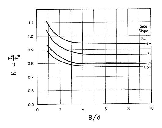
Channel Side Shear Stress To Bottom Shear Stress Ratio,  ${\rm K}_1$ .
