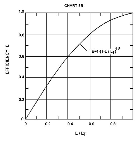
Curb-opening and Slotted Drain Inlet Interception Efficiency.
