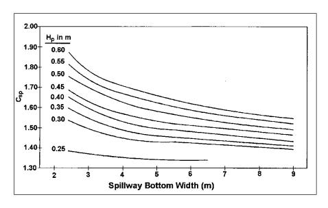
Figure 8-18a. Discharge coefficients for emergency spillways, SI units.
