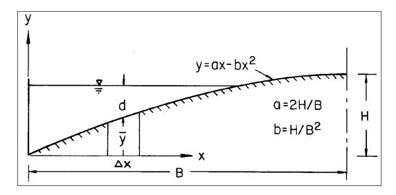
Figure B-2. Properties of a parabolic curve.
