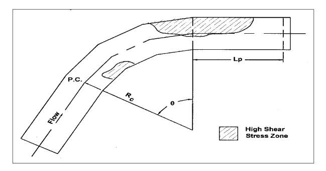
Figure 5-5. Shear stress distribution in channel bends.
