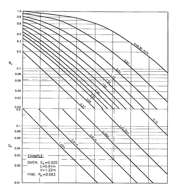
Grate Inlet Side Flow Intercept Efficiency.
