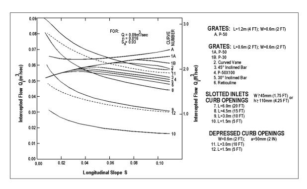
Figure 4-11. Comparison of inlet interception capacity, slope variable.
