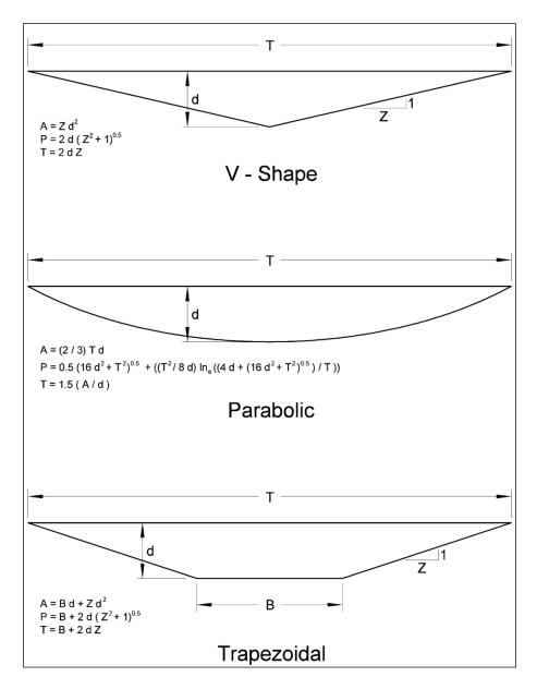
Figure 5-6. Channel geometries.
