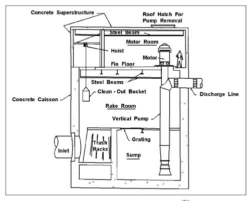
Figure 9-1. Typical wet-pit station. (51)
