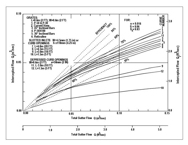
Figure 4-12. Comparison of inlet interception capacity, flow rate variable.
