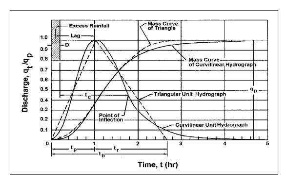
Figure 3-7. Dimensionless curvilinear SCS synthetic unit hydrograph and equivalent triangular hydrograph.
