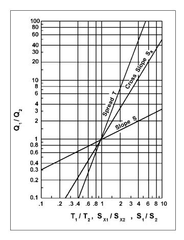
Figure 4-3. Relative effects of spread, cross slope, and longitudinal slope on gutter capacity.
