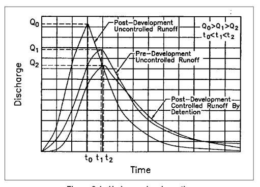
Figure 8-1. Hydrograph schematic.
