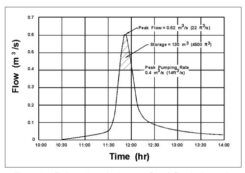
Figure 9-5. Estimated required storage from inflow hydrograph.
