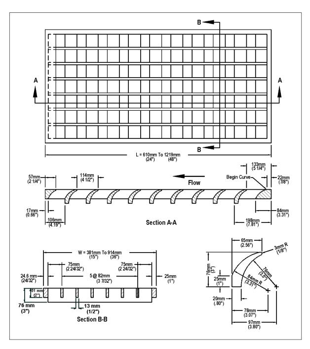
Figure 4-7. Curved vane grate.
