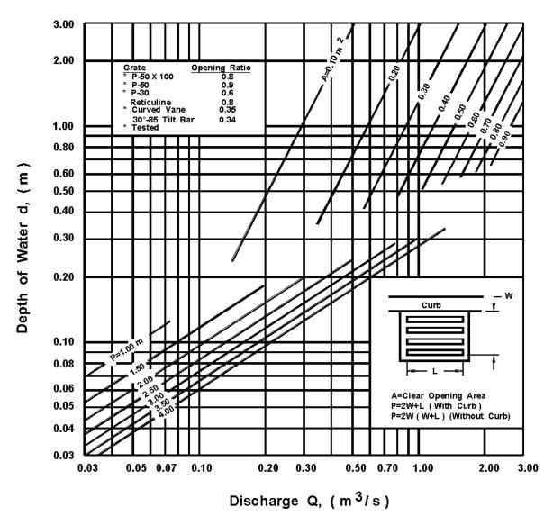
Grate Inlet Capacity in Sump Conditions.
