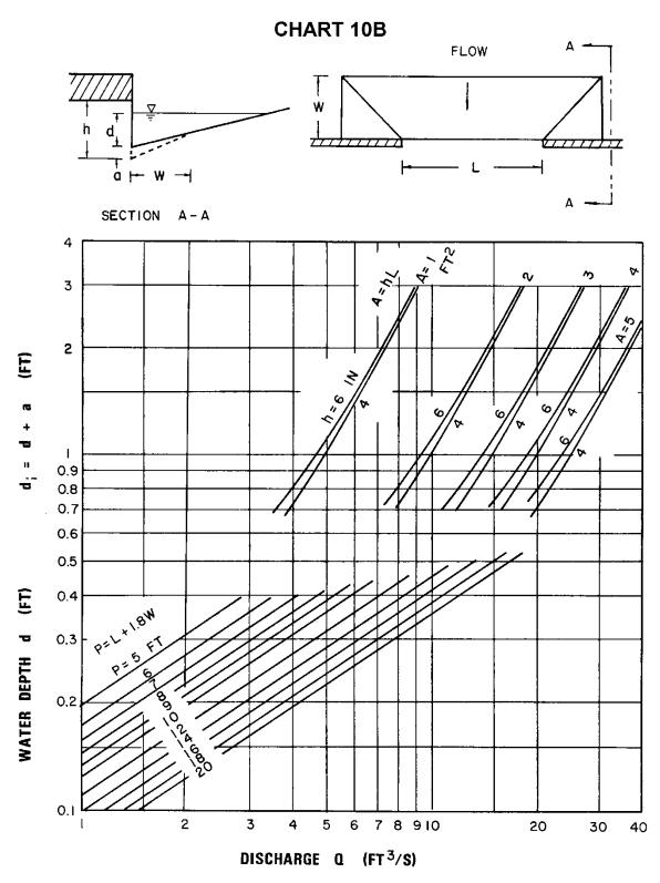
Depressed Curb-opening Inlet Capacity in Sump Locations - English Units
