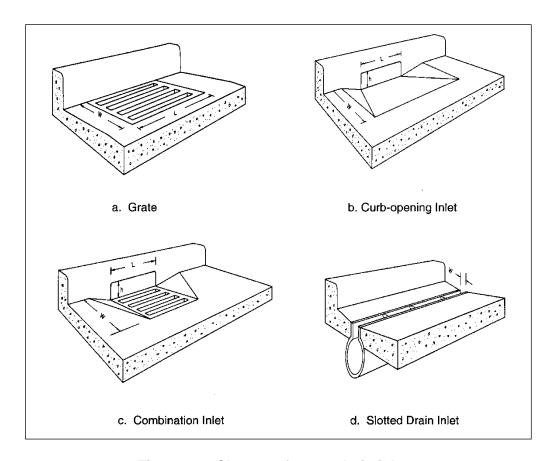
Figure 4-4. Classes of storm drain inlets.
