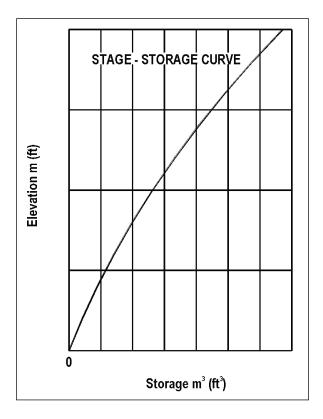
Figure 8-6. Stage-storage curve.
