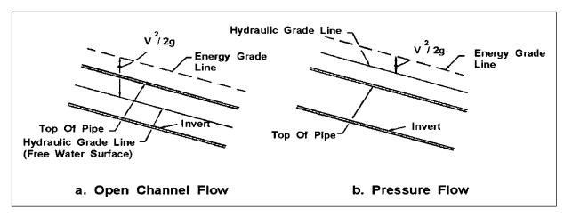
Figure 7-2. Hydraulic and energy grade lines in pipe flow.
