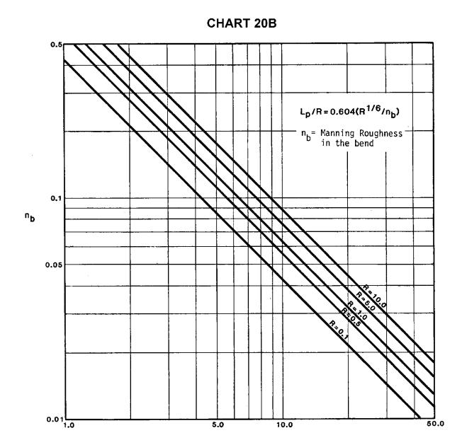
$$L_p/R$$  Protection Length,  $L_p$  , Downstream of Channel Bend  $^{\mbox{\tiny (11)}}$  - English Units
