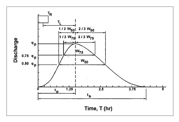
Figure 3-6. Snyder synthetic hydrograph definition.
