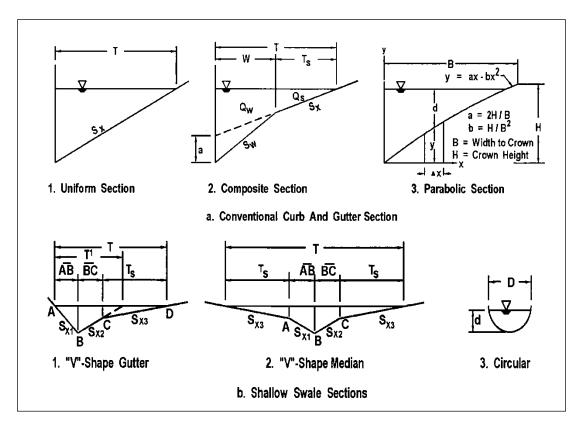
Figure 4-1. Typical gutter sections.
