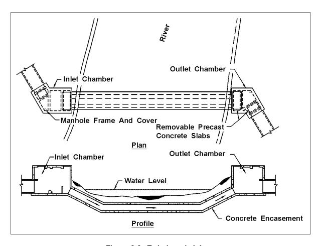
Figure 6-6. Twin-barrel siphon.
