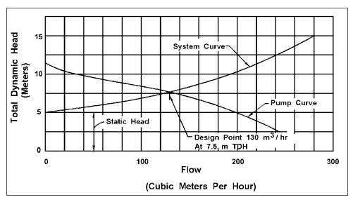
Figure 9-3. System head curve. (51)
