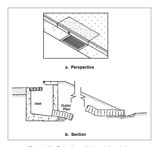
Figure 4-24. Embankment inlet and downdrain.
