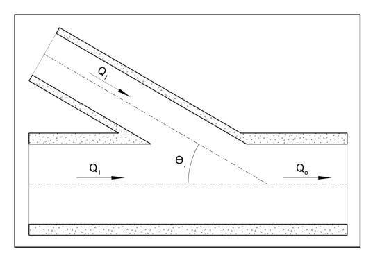
Figure 7-4. Interior angle definition for pipe junctions.
