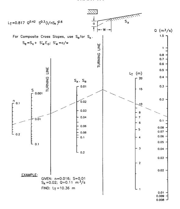
Curb Opening & Slotted Drain Inlet Length for Total Interception
