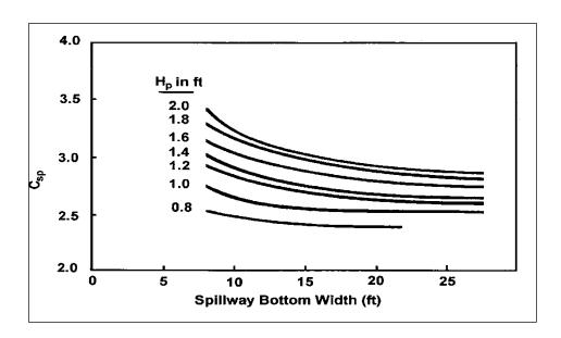
Figure 8-18b. Discharge coefficients for emergency spillways, English units.
