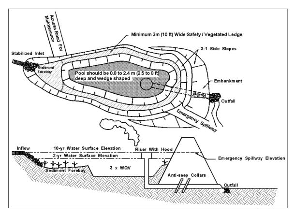
Figure 10-2. Typical wet pond schematic.
