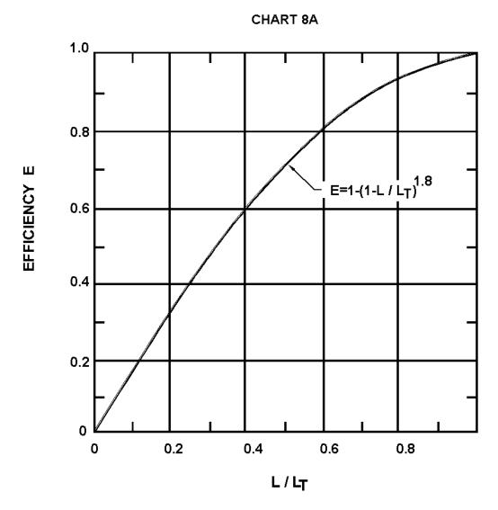
Curb-opening and Slotted Drain Inlet Interception Efficiency.
