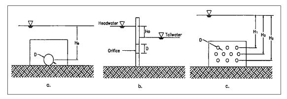
Figure 8-12. Definition sketch for orifice flow.
