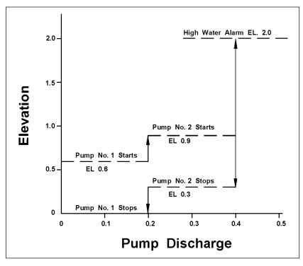
Figure 9-8. Stage-discharge curve.
