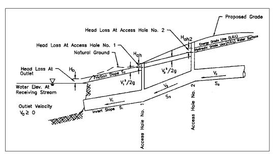
Figure 7-9. Energy and hydraulic grade line illustration.
