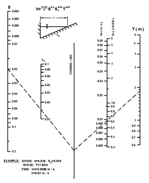
Velocity In Triangular Gutter Sections.
