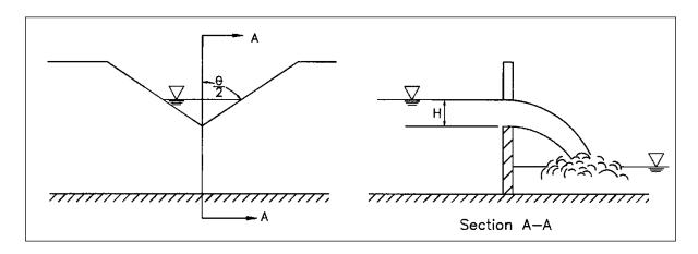
Figure 8-15. V-notch weir.
