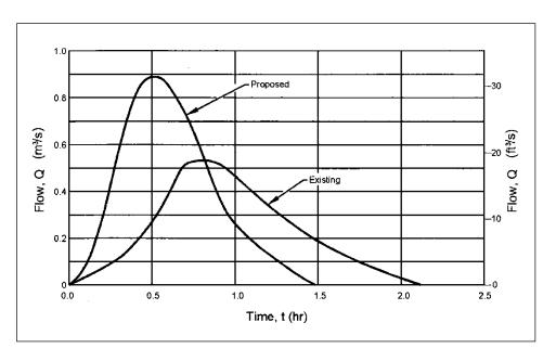
Figure 3-9. USGS Nationwide Urban Hydrograph for existing (unimproved) and proposed (improved) conditions.
