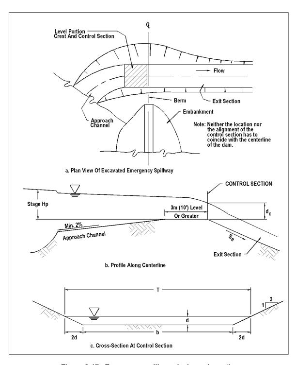
Figure 8-17. Emergency spillway design schematic.
