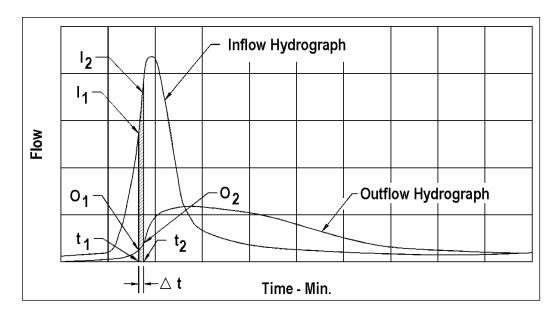
Figure 8-20. Routing hydrograph schematic.
