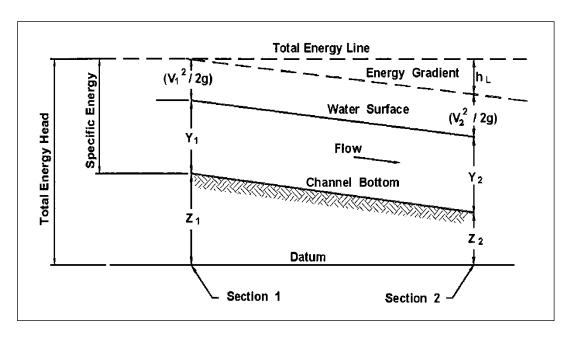
Figure 5-1. Total energy in open channels.
