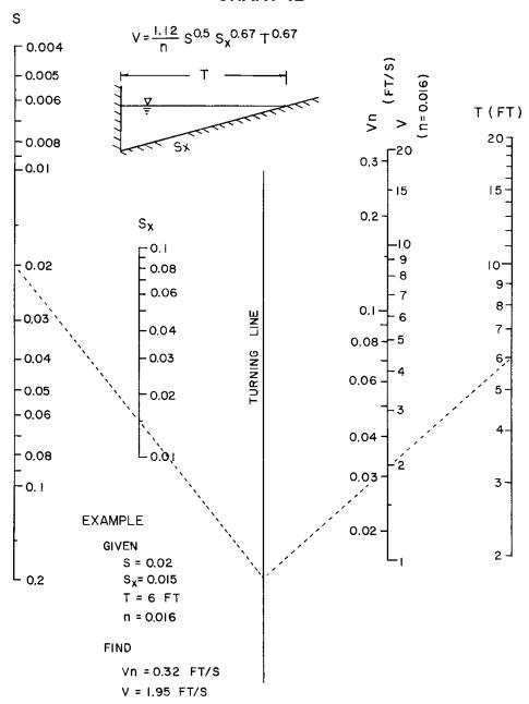
Velocity in Triangular Gutter Sections - English Units
