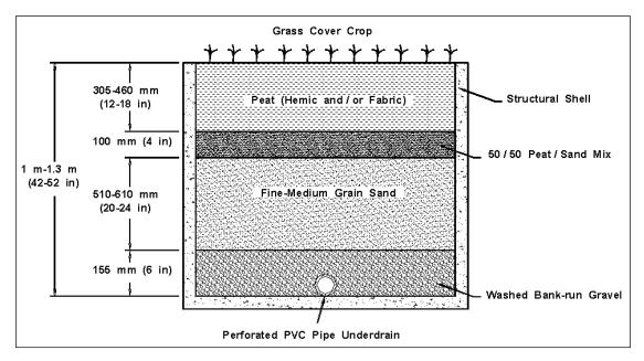
Figure 10-6. Cross-section schematic of peat-sand filter.
