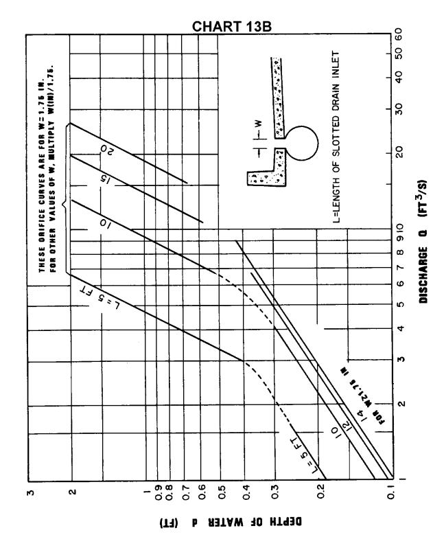
Slotted Drain Inlet Capacity in Sump Locations - English Units
