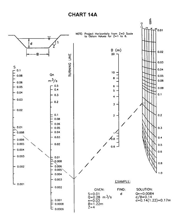
Solution to Manning's Equation for Channels of Various Side Slopes.
