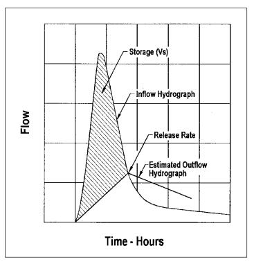
Figure 8-3. Estimating required storage hydrograph method.
