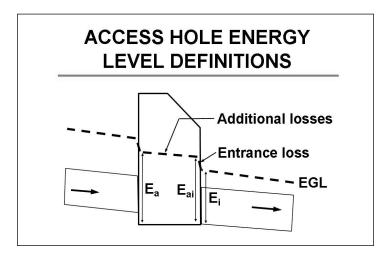
Figure 7-5. Definition sketch for FHWA access hole method.
