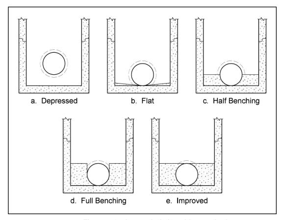
Figure 7-6. Access hole benching methods.
