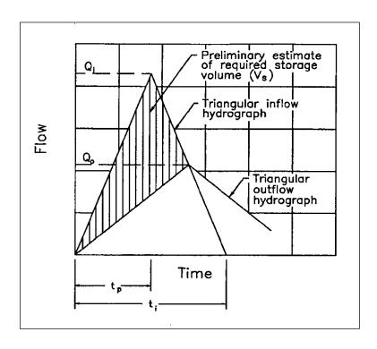
Figure 8-4. Triangular hydrograph method.
