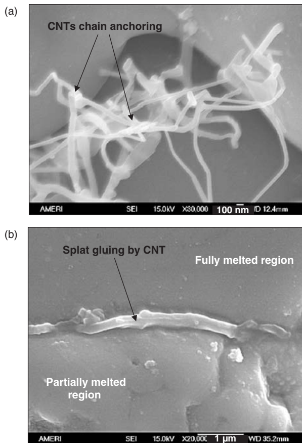
Fig. 7. SEM image of AC-B coating depicting (a) fusion of CNTs in \text{Al}_2\text{O}_3 , and (b) alignment of CNTs along splat interface.
