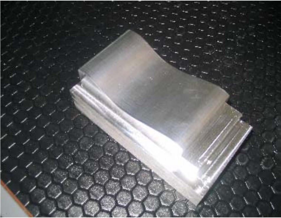
Figure 2. The completed part after the machining operation.
