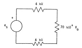
The output voltage is given by the voltage divider equation
