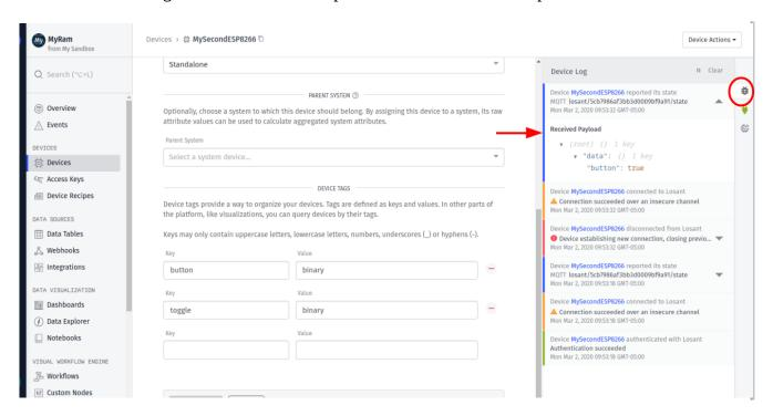
Every time the button is pressed, the firmware is publishing the state { "button": true } to Losant. Currently, this firmware only reports when the button goes to true, it does not report the button going back to false. So if you hold the button down for a long time, it will only report when the button is initially pressed.
