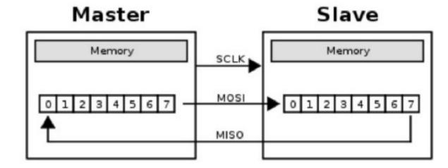
SPI is used to talk to a variety of peripherals, such as
