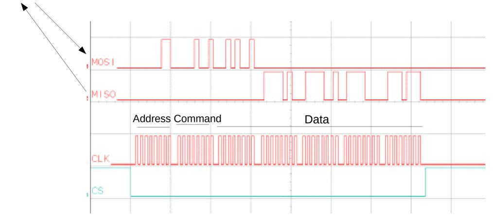
3. The master keeps cycling the clock, bits are traded, and after eight bits, both sides read in the received data and queue up the next byte for transmission.
