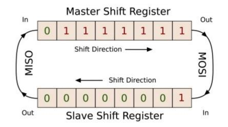
It's this simplicity that makes SPI fast. While asynchronous serial communications can run in the hundred-of-thousands of bits per second, SPI is usually good for ten megabits per second or more.
