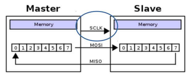
A typical hardware setup using two <u>shift registers</u> to form an inter-chip <u>circular buffer</u>
