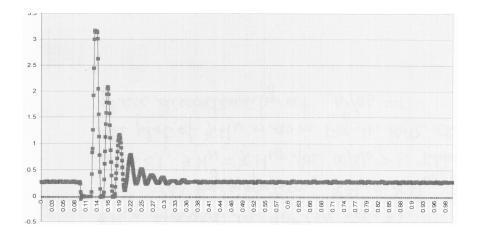
The waveform was "cleaned up" and translated into the MATLAB plot shown below. This waveform can be subjected to graphical analysis to calculate the values of resonant frequency and damping ratio (see text, section 1.10).
