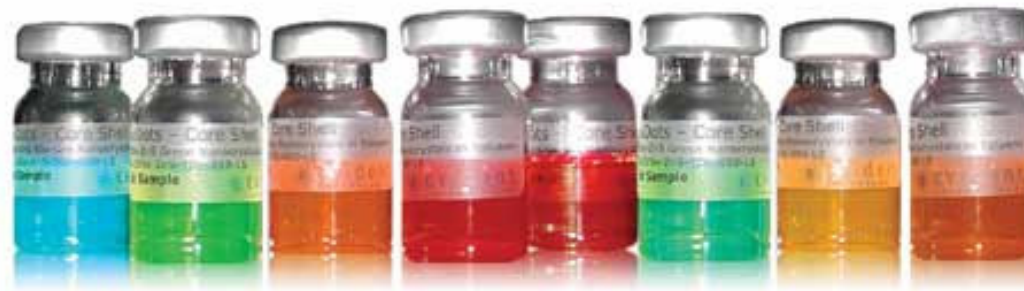
CdSe core with ZnS shell QDs
