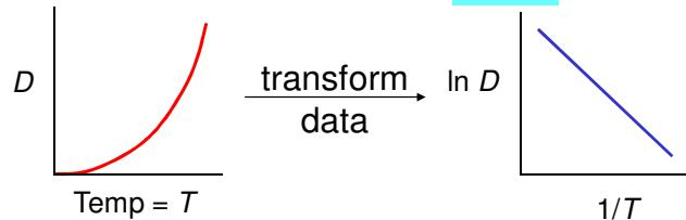
$$\ln D_2 = \ln D_0 - \frac{Q_d}{R} \left( \frac{1}{T_2} \right) \quad \text{and} \quad \ln D_1 = \ln D_0 - \frac{Q_d}{R} \left( \frac{1}{T_1} \right)$$
