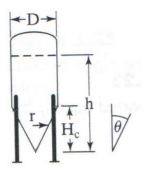
If height of solid is less than height of conical section:
