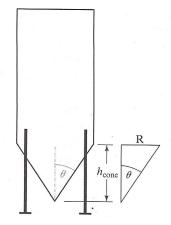
To calculate the volume of the contents, you use the formula for a cone along as the height of product, h, is less than the height of the conical section  $h_{\text{cone}}$ :
