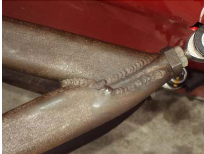
Figure 11 Welding Sample 1, approved
