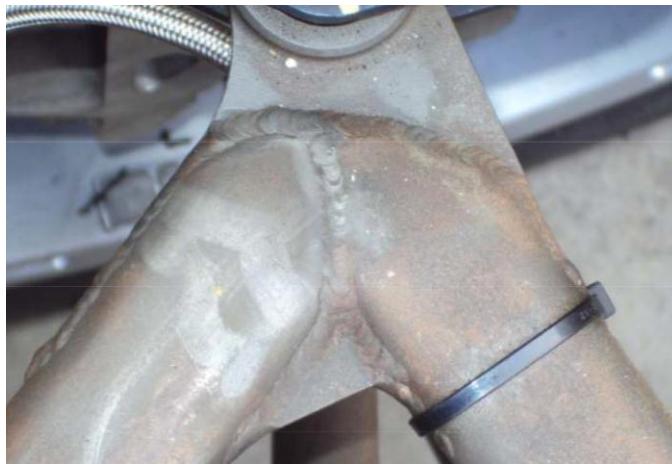
Figure 12 Welding Sample 2, approved
