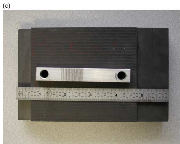
Fig. 4. Experimental set-up: (a) diagram of the experimental set-up; (b) picture of the set-up; (c) POCO workpiece and aluminium test piece with slots.
