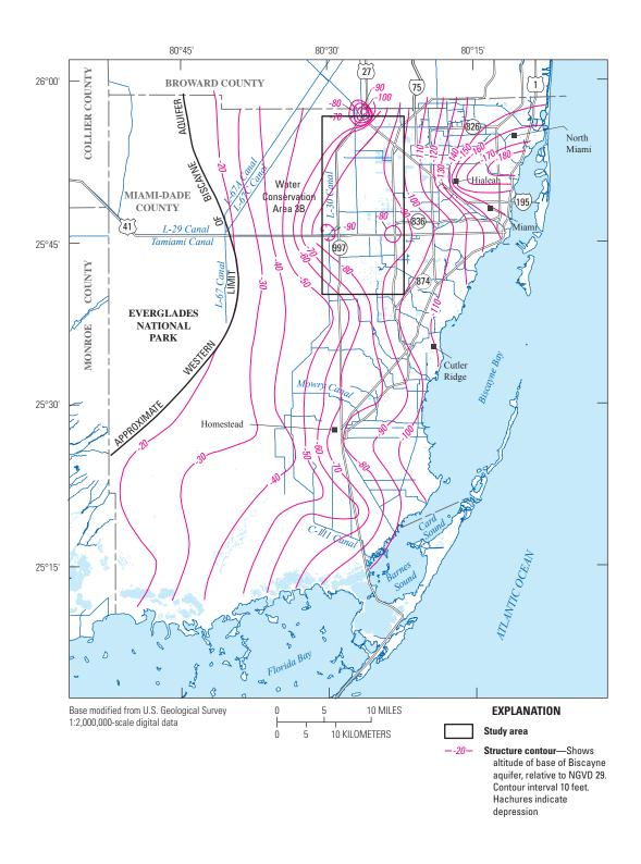
**Figure 6.** Altitude of the base of the Biscayne aquifer and its western extent throughout most of Miami-Dade County (Fish and Stewart, 1991).
