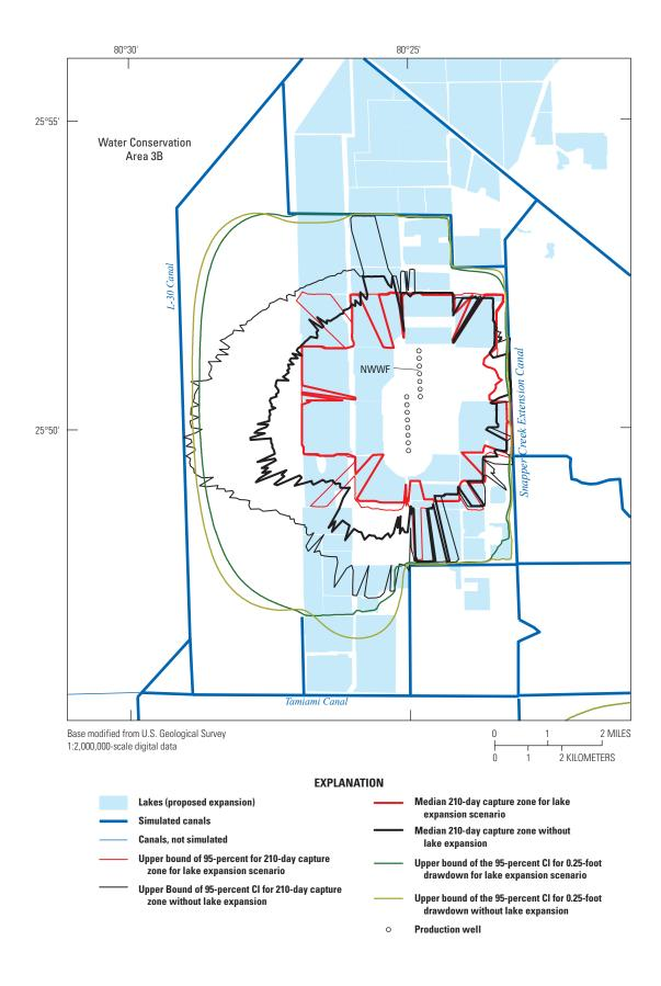
Figure 49. Median and upper bound of the 95-percent confidence intervals (CI) for the 210-day capture zones and upper bound of the 95-percent CI for the 0.25-foot drawdown for the Northwest Well Field (NWWF) for steady-state dry conditions for the lake expansion scenario and without lake expansion. Area shown is Base map 4 (fig. 1). 106
