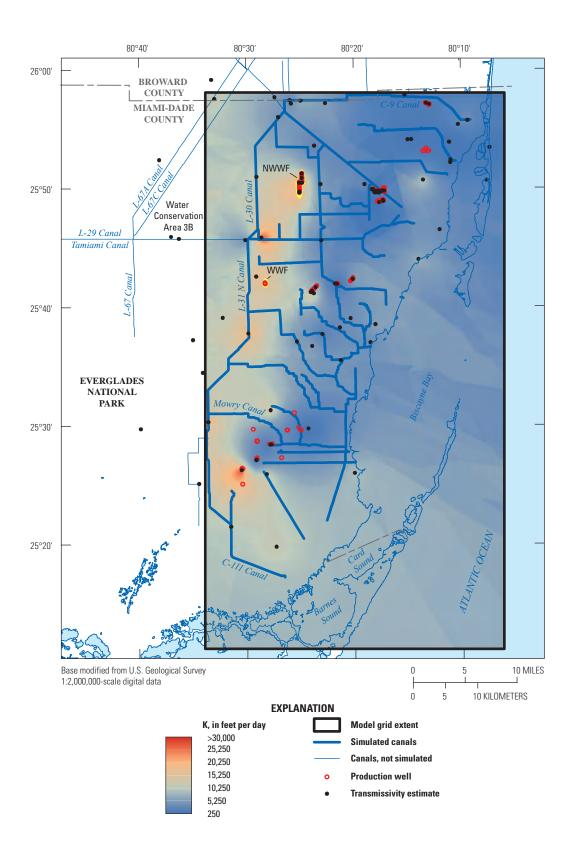
**Figure 11.** Hydraulic conductivity field for the base-case simulation and locations of transmissivity estimates derived from aquifer performance tests. Area shown is Base map 1 (fig. 1).
