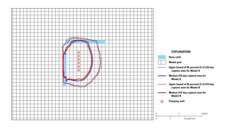
Figure 1–4. . Median and upper bound of 95-percent confidence interval (CI) for 210-day capture zones for Model A and Model B.
