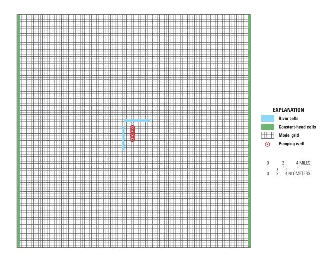
**Figure 1–2.** Model grid, locations of constant-head cells, river cells and pumping wells for Model A and Model B.
