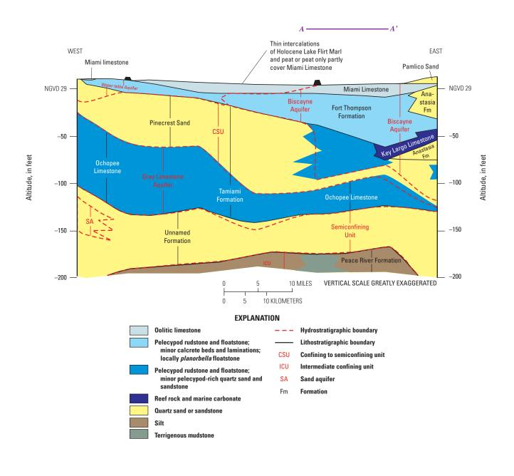
**Figure 4.** Hydrogeologic cross section with subset section *A–A'*. Modified from Reese and Cunningham (2000). Location of subset cross section shown in fig. 2.
