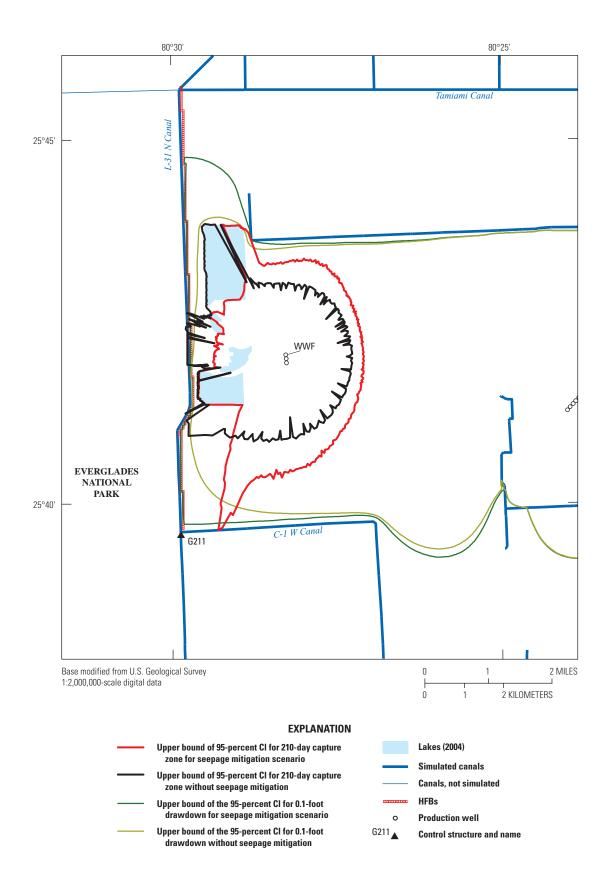
**Figure 46.** Upper bound of the 95-percent confidence intervals (CI) for the 210-day capture zones and upper bound of the 95-percent CI for the 0.1-foot drawdown for the West Well Field (WWF) for steady-state, dry conditions for seepage mitigation scenario and without seepage mitigation. Area shown is Base map 5 (fig. 1).
