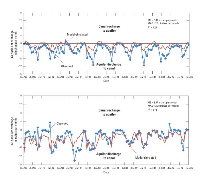
**Figure 16.** Monthly model-simulated (red) and observed (blue) net exchange for composite C-4 and C-6 basins, and mean error (ME), mean absolute error (MAE) and the coefficients of determination (R<sup>2</sup>) for simulated versus observed net exchange for each basin.
