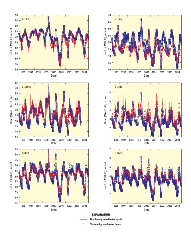
**Figure 5–1.** Daily observed and model-simulated water levels for monitoring wells in the study area not shown in figure 13.
