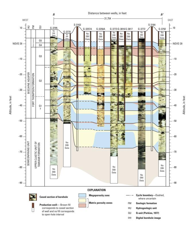
**Figure 5**. Hydrogeologic cross section B–B′ across central part of the study area, including the Northwest Well Field (modified from Renken and others, 2008). Location of cross section shown in fig. 2.
