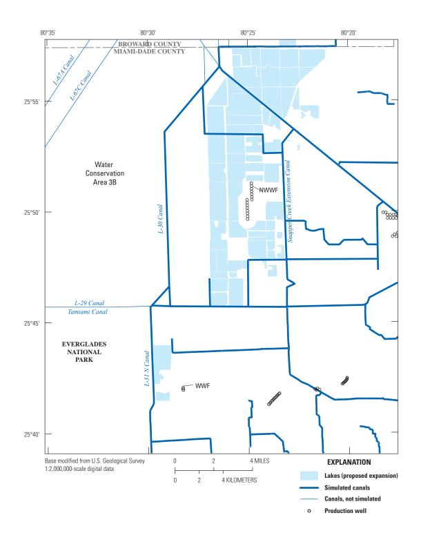
**Figure 48.** Locations of existing lakes, projected expansion of existing lakes and new proposed lakes for lake-expansion scenario. Area shown is Base map 2 (fig. 1). NWWF is Northwest Well Field. WWF is West Well Field.
