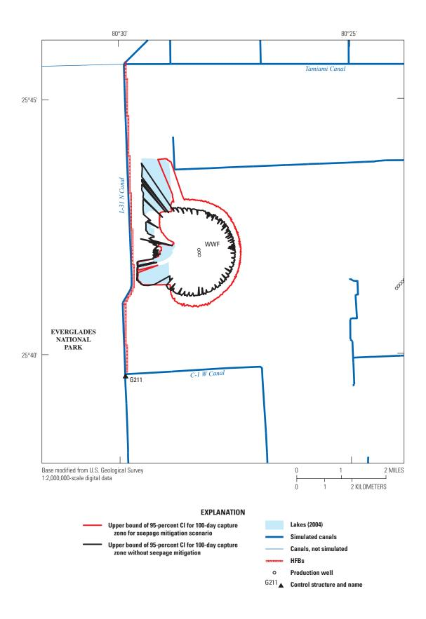
**Figure 47.** Upper bound of the 95-percent confidence intervals (CI) for the 100-day capture zones for the West Well Field (WWF) for steady-state, dry conditions for seepage mitigation scenario and without seepage mitigation. Area shown is Base map 5 (fig. 1).
