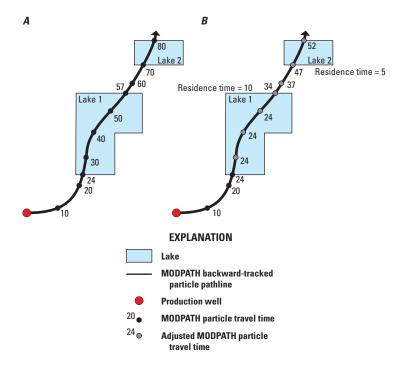
**Figure 6–1.** Backward-tracked particle pathlines from a pumping well through lakes (*A*) without residence-time post-processing, (*B*) with residence-time post-processing.
