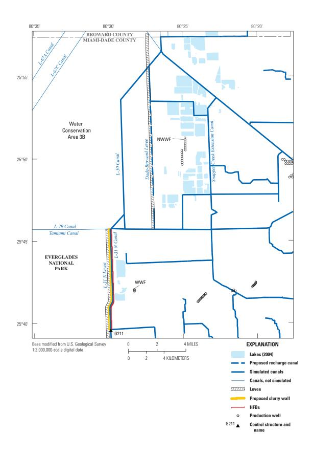
**Figure 44.** Locations of the recharge canal west of the Northwest Well Field (NWWF), the proposed slurry wall between the L-31N Levee and the L-31N Canal, and the Horizontal Flow Barriers (HFBs) west of the West Well Field (WWF) for Scenario 1. Area shown is Base map 2 (fig. 1).
