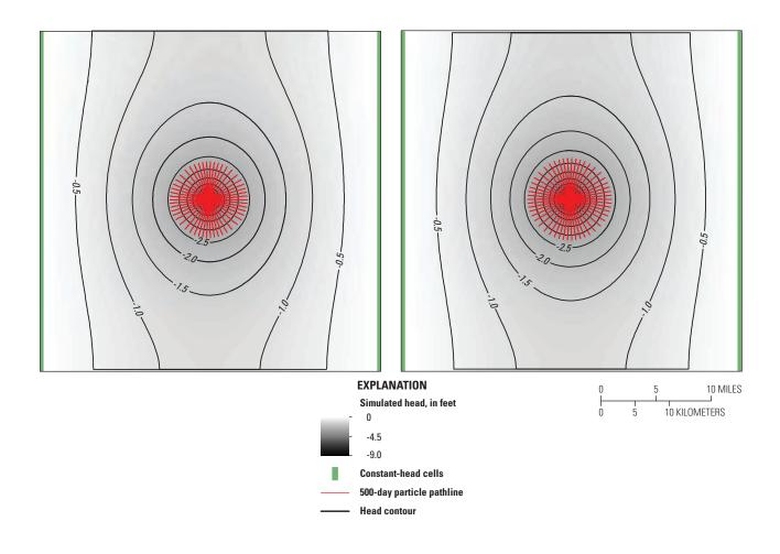
Figure 1–1. Simulated 500-day particle pathlines and head contours for one-layer conceptual Model A (left) and three-layer conceptual Model B (layer 2) (right).
