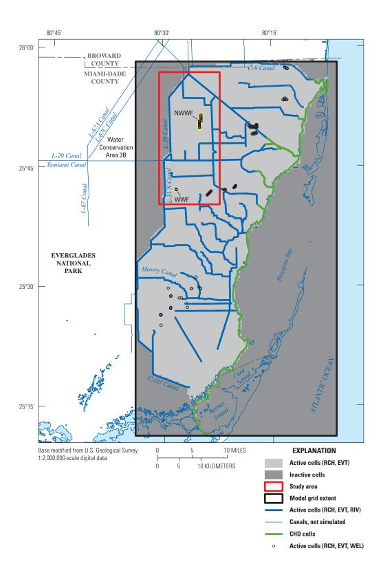
**Figure 9.** Location of active and inactive model cells, and type of MODFLOW boundary condition. [RCH = Recharge Package, EVT = Evapotranspiration Package, RIV = River Package, CHD = Time-Variant Specified-Head Package, and WEL = Well Package]. Area shown is Base map 1 (fig. 1). NWWF is Northwest Well Field. WWF is West Well Field.
