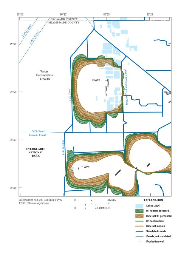
**Figure 42.** Median and 95-percent confidence intervals (CI) for 0.1-foot and 0.25-foot drawdowns for the Northwest Well Field (NWWF) and West Well Field (WWF) for steady-state, average conditions. Area shown is Base map 2 (fig. 1).
