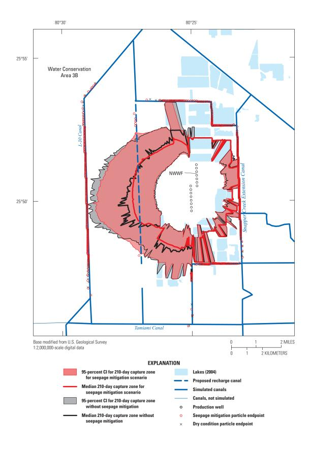
**Figure 45.** Median and 95-percent confidence intervals for the 210-day capture zones for the Northwest Well Field (NWWF) for steady-state, dry conditions for seepage mitigation scenario and without seepage mitigation, and final particle endpoints for both conditions beyond 210 days. Area shown is Base map 4 (fig. 1).
