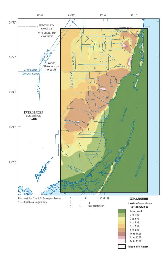
Figure 10. Altitude of the top of the Biscayne aquifer model. Area shown is Base map 1 (fig. 1).
