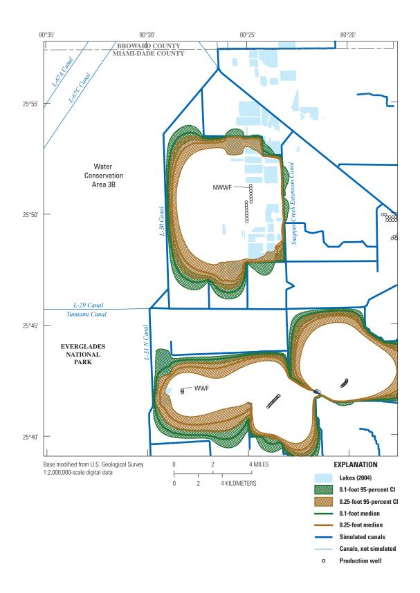
**Figure 43.** Median and 95-percent confidence intervals (CI) for 0.1-foot and 0.25-foot drawdowns for the Northwest Well Field (NWWF) and West Well Field (WWF) for steady-state, wet conditions. Area shown is Base map 2 (fig. 1).
