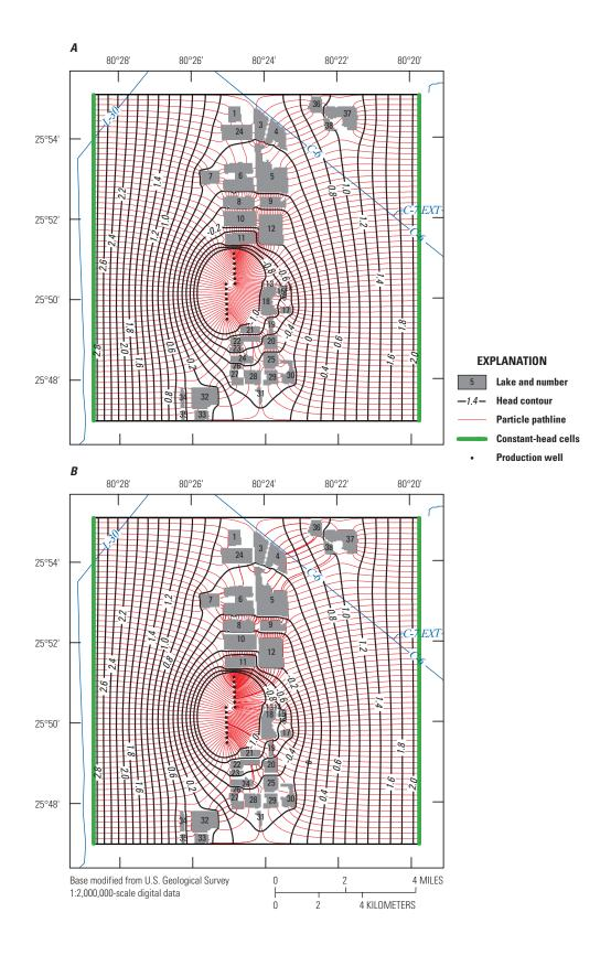
**Figure 4–1.** Simulated steady-state groundwater head and backward-tracked particle pathlines for (*A*) the model representing lakes with high hydraulic conductivity and (*B*) the model using the LAK Package to represent lakes. Lake numbers correspond to data in Table 4-1.
