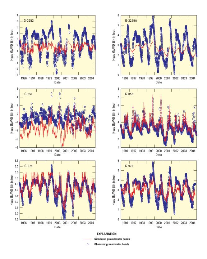
Figure 13. Daily observed and model-simulated water levels for selected monitoring wells in the study area.
