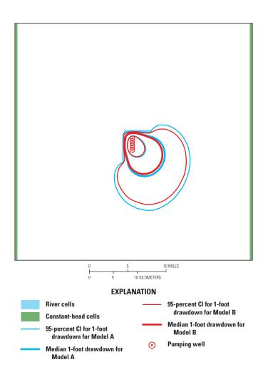
**Figure 1–3.** Median and 95-percent confidence intervals (CI) for 1-foot drawdown for Model A and Model B.
