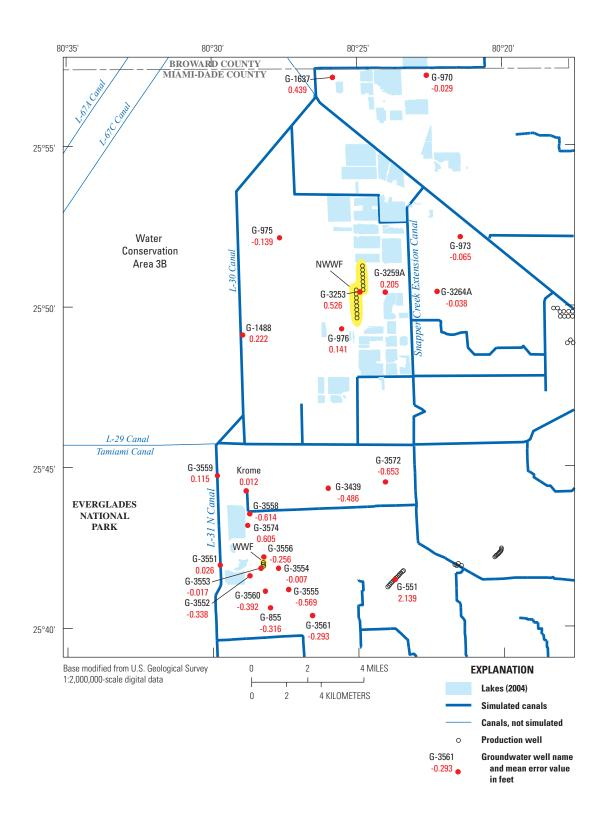
**Figure 14.** Locations of groundwater observation data used to calibrate model and mean error calculated from observed and simulated daily water levels. Area shown is Base map 2 (fig. 1). NWWF is Northwest Well Field. WWF is West Well Field.
