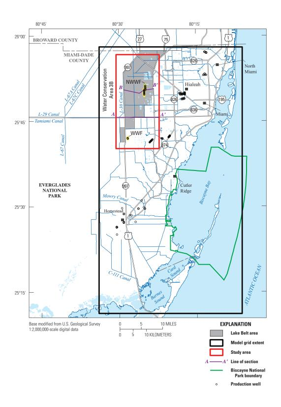
**Figure 2**. Model grid extent, study area, hydrogeologic sections A–A′ and B–B′, location of production well fields and location of canals, southeastern Florida. Area shown is Base map 1 (fig. 1). NWWF is Northwest Well Field. WWF is West Well Field.
