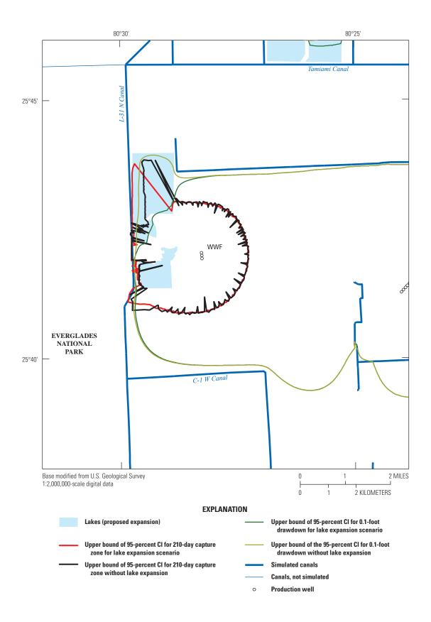
**Figure 50.** Upper bound of the 95-percent confidence intervals (CI) for the 210-day capture zones and upper bound of the 95-percent CI for the 0.1-foot drawdown for the West Well Field (WWF) for steady-state, dry conditions for the lake expansion scenario and without lake expansion. Area shown is Base map 5 (fig. 1).
