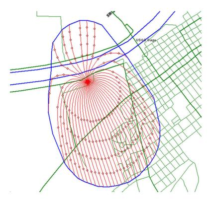
Figure 5.18: 5-year capture zones including resistance of Wabash River (c=14.3 days,  $\delta=1$  ft, widthB=615 ft
