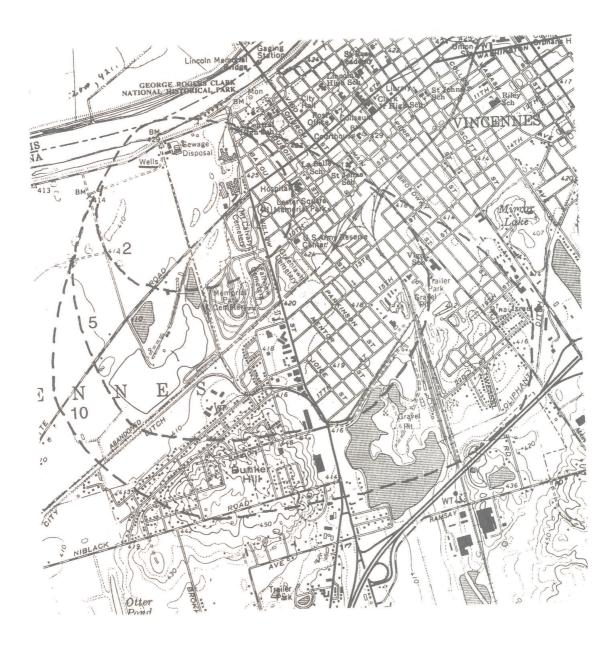
Figure 5.19: Composite time of travel capture zones with 2-,5-, and 10-year isochrones for the city well field using the full-feature analytic element model GFLOW (after [Haitjema,1995]).
