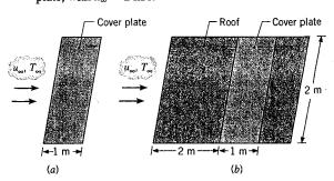
(a) What is the rate of convective heat loss from the plate?
