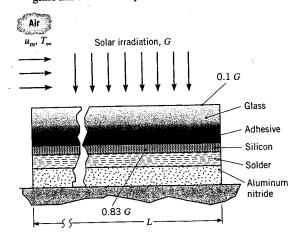
(a) Consider an L = 1 m long, w = 0.1 m wide solar cell that is placed on an insulated surface. Determine the silicon temperature and the electric power produced by the solar cell for an air velocity of 4 m/s parallel to the long direction, with air and surroundings temperatures of 25°C. The solar irradiation is 700 W/m². The boundary layer is tripped to a turbulent condition at the leading edge of the panel.
