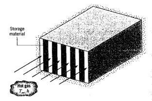
Each layer of the storage material is an aluminum slab of width W=0.05 m, which is at an initial temperature of 25°C. Consider conditions for which the storage unit is charged by passing a hot gas through the passages, with the gas temperature and the convection coefficient assumed to have constant values of  $T_{\infty}=600$ °C and  $h=100 \text{ W/m}^2 \cdot \text{K}$  throughout the channel. How long will it take to achieve 75% of the maximum possible
