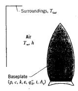
If an approximately uniform heat flux of  $q_h^n = 1.25 \times 10^4 \text{ W/m}^2$  is applied to the inner surface of the base plate and the convection coefficient at the outer surface is  $h = 10 \text{ W/m}^2 \cdot \text{K}$ , estimate the time required for the plate to reach a temperature of 135°C. *Hint:* Numerical integration is suggested in order to solve the problem.
