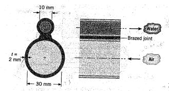
11.29 A twin-tube, counterflow heat exchanger operates with balanced flow rates of 0.003 kg/s for the hot and cold airstreams. The cold stream enters at 280 K and must be heated to 340 K using hot air at 360 K. The average pressure of the airstreams is 1 atm and the maximum allowable pressure drop for the cold air is 10 kPa. The tube walls may be assumed to act as fins, each with an efficiency of 100%.
