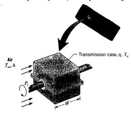
If the transmission efficiency is  $\eta = 0.93$  and air flow over the case corresponds to  $T_x = 30^{\circ}\text{C}$  and  $h = 200 \text{ W/m}^2 \cdot \text{K}$ , what is the surface temperature of the transmission?
