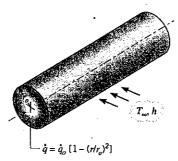
Obtain an expression for the total rate at which energy is generated in a unit length of the container. Use this result to obtain an expression for the temperature  $T_s$  of the container wall.
